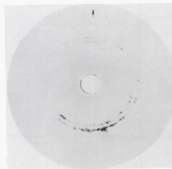
(f) Crept 149 minutes to rupture at about 33-percent strain.
