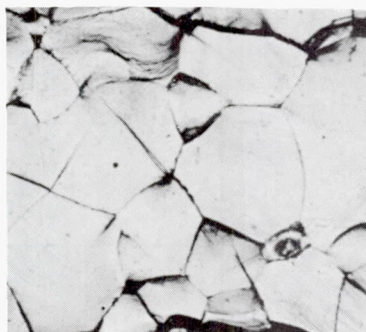
(c) 2-percent-copper alloy; 300° C; 2400-psi stress; 13.3-percent strain; 3,261 minutes.
