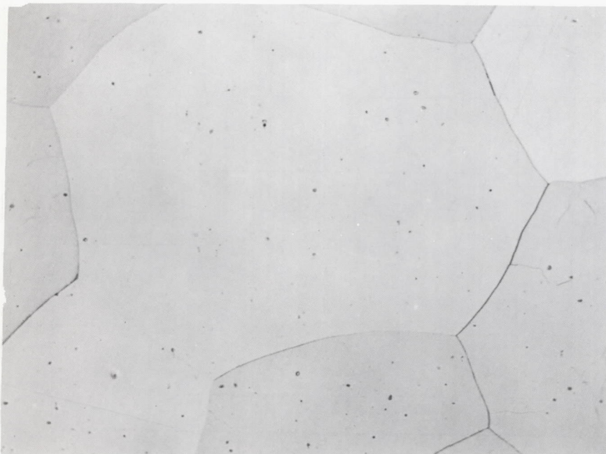
(b) Polished and etched surface; same area as above. L-57-2576 New grain size is 1.06 grains per millimeter.
