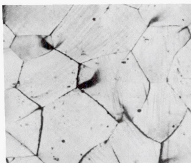
(e) 2-percent-copper alloy; 200° C; 7,500-psi stress; 11.1-percent strain; 3,428 minutes.
