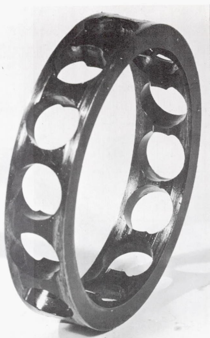
(a) Bearing 1009. Cage wear resulting from several oil-interruption tests.
