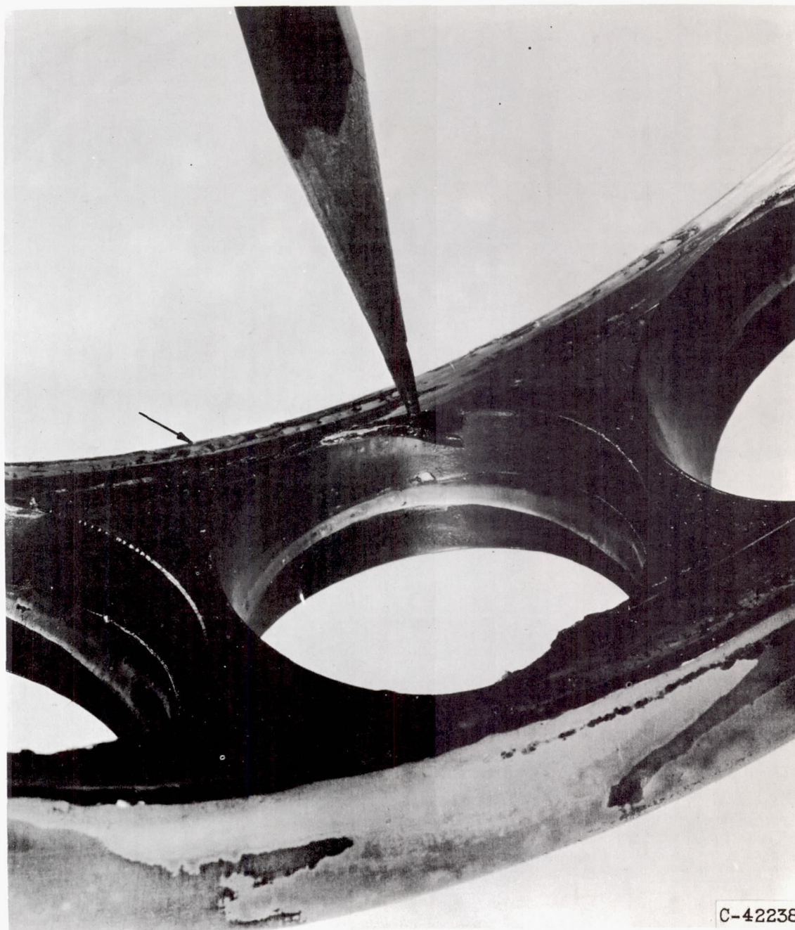
(g) Bearing 1005A. Cage locating surface and pocket wear resulting from an oil-interruption test.
