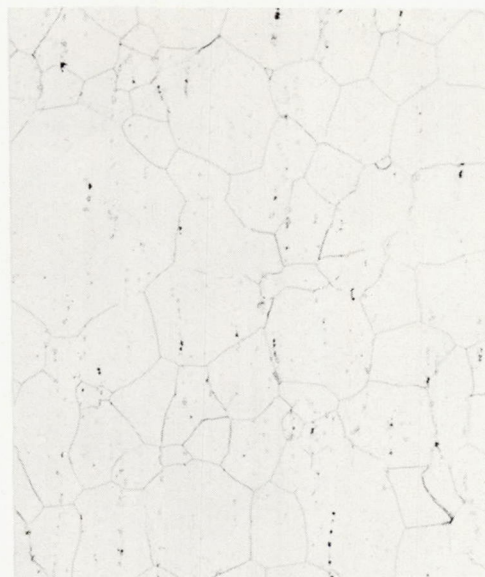
(b) Heat V-12 with 0.0089 percent boron and less than 0.01 percent zirconium.
