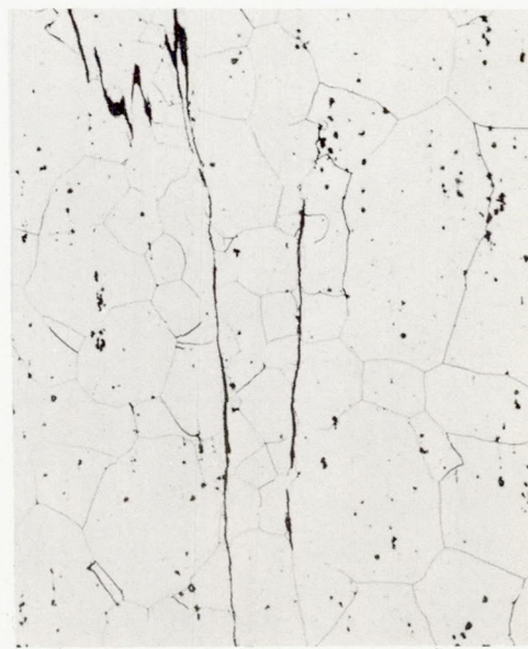
(d) Heat V-18 with 0.0069 percent boron and 0.09 percent zirconium.
