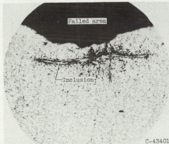
(k) Fatigue failure caused by inclusions in SAE 52100. X250.
