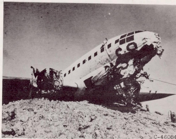
(c) Angle of impact, 29°; impact speed, 97 mph.
