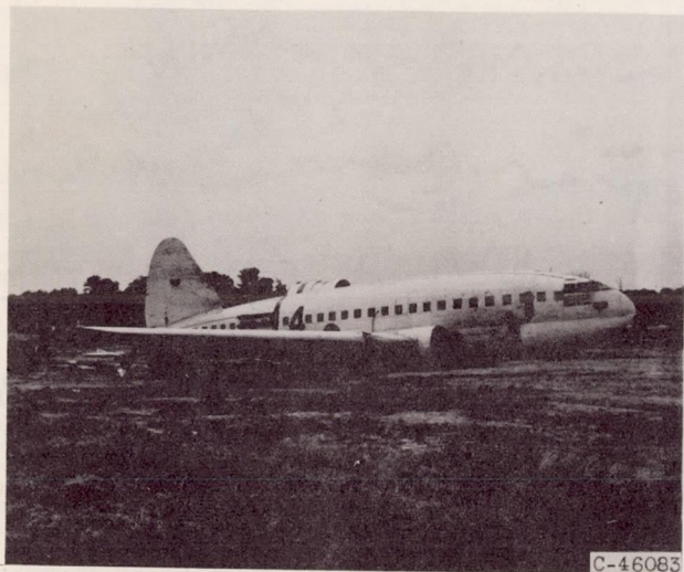
(a) Angle of impact, 5°; impact speed, 81 mph.
