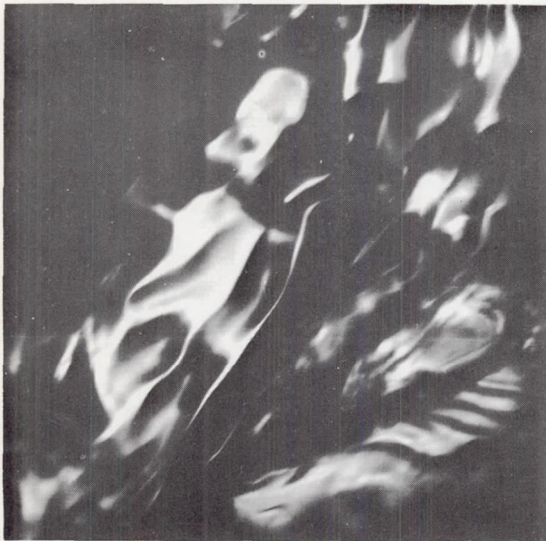
(b) Sheet and wave formation, 1 inch from point of impingement (zone I); x21.
