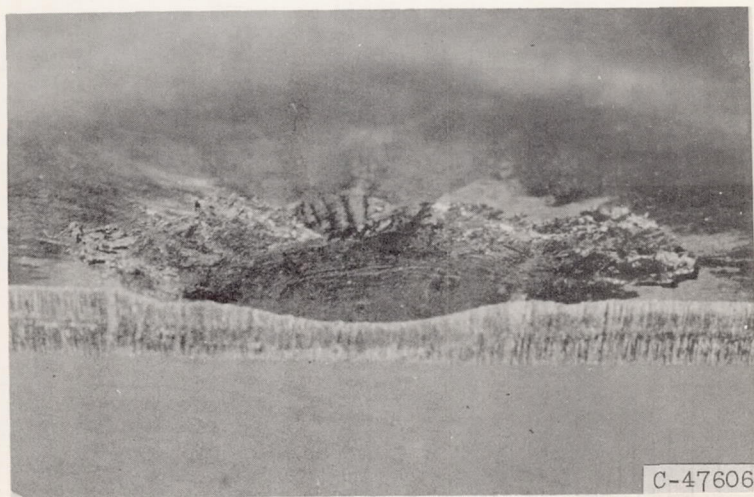
Figure 8. - Cross section through center of crater produced by laboratory discharge to 1/8-inch-thick aluminum plate.
