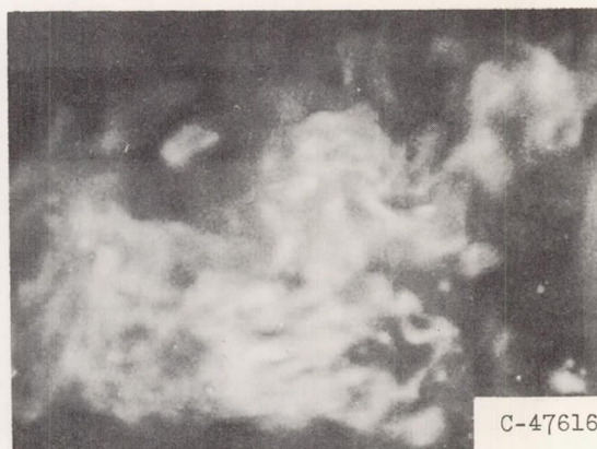
Figure 10. - Photographic sequence of sample fuel-tank ignition by artificial-lightning discharge.
