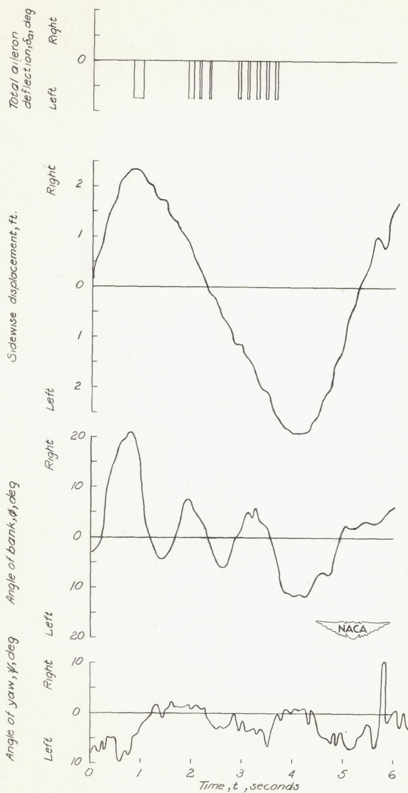
Figure 7(b).- Time histories of the lateral motions of the model for mass condition C_2 .
