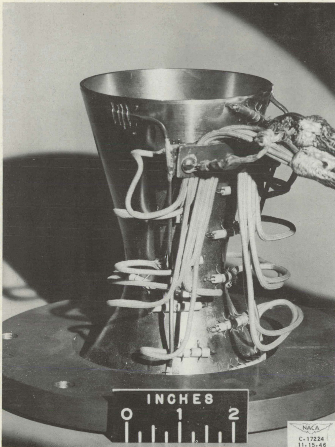
Figure 4. - Thin-wall stainless-steel nozzle showing part of thermocouple installation.
