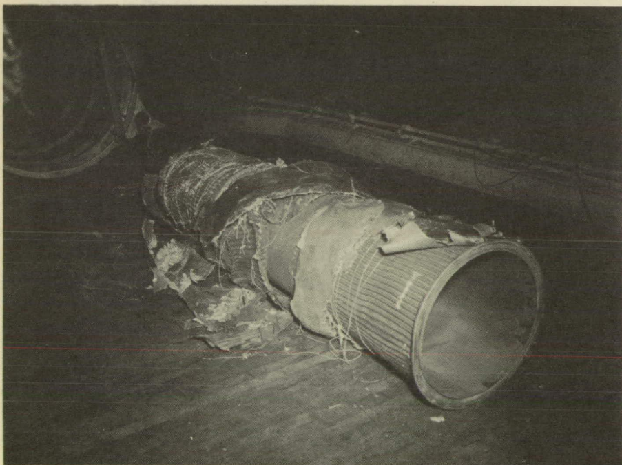
Figure 32.- Views showing damage to fuselage, tail pipe, and tail-pipe insulation of I-40 jet-propulsion engine.
