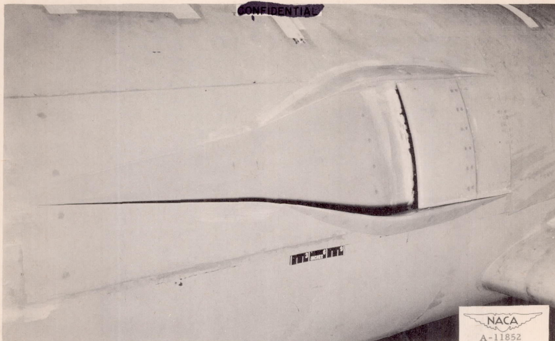
(a) 7^\circ ramp, standard divergence.
