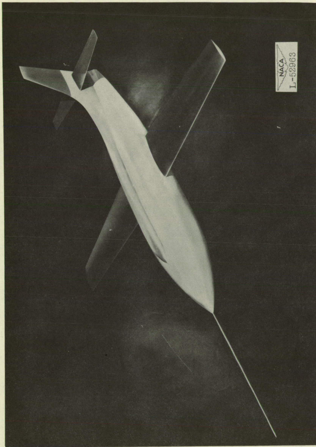
Figure 1.- Three-quarter front view of \frac{1}{4} -scale model of the Bell XS-1 airplane used in free-fall test.
