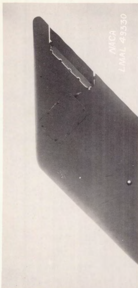
Figure 2.- RM-1 wing-aileron combination.
