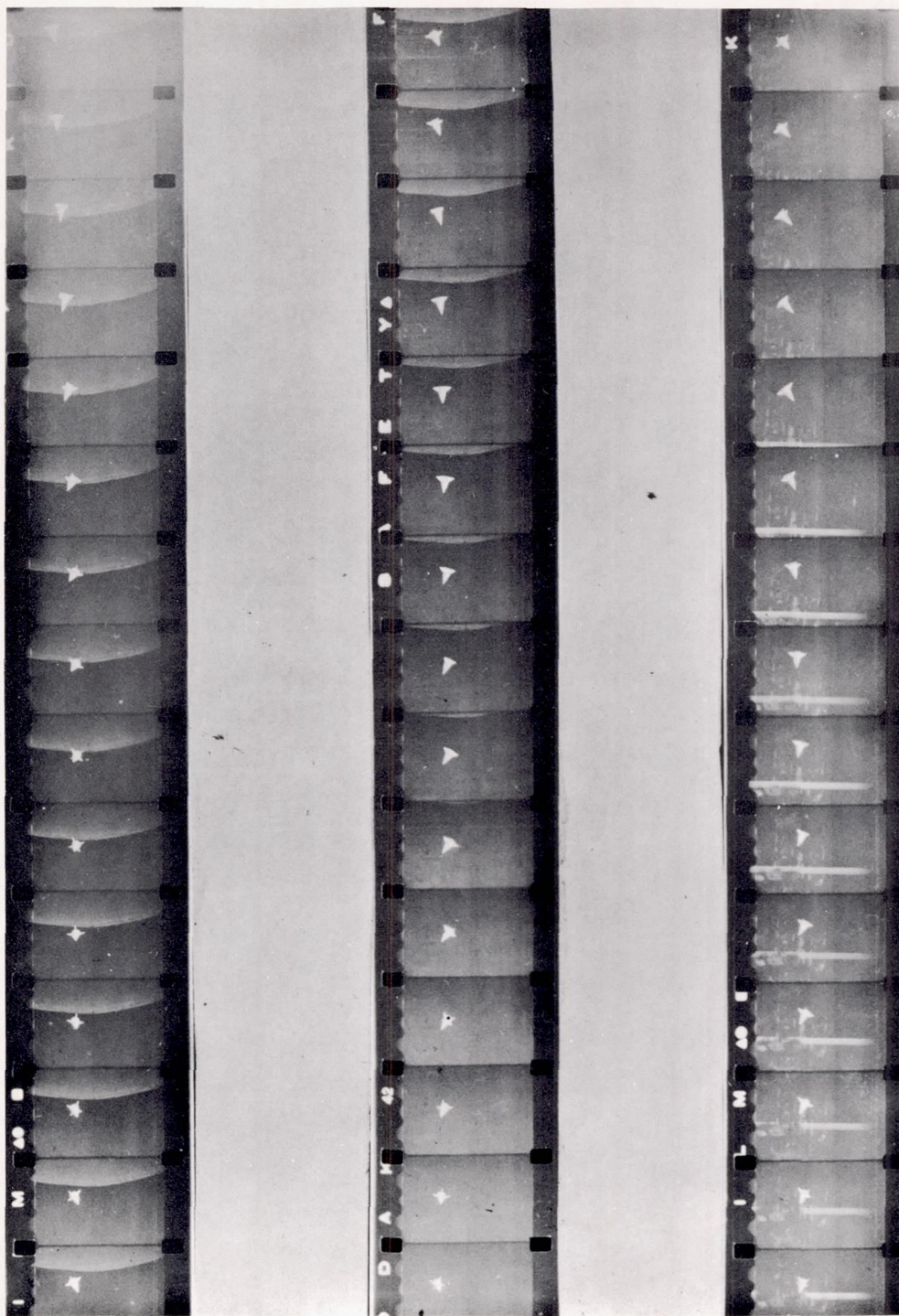
Figure 12.- Moving picture strip of tests of the \frac{1}{12} -scale model of the jettisonable nose section of the D-558, phase II, airplane with the center of gravity at 0.624L and fins II-4 installed. The model is shown damping applied rotation and descending in a stable nose-down attitude in the Langley 20-foot free-spinning tunnel.
