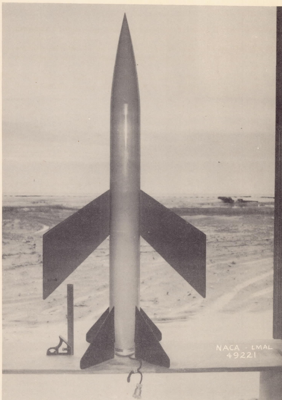
Figure 1.- The test body with swept-back wing having inverse taper.
