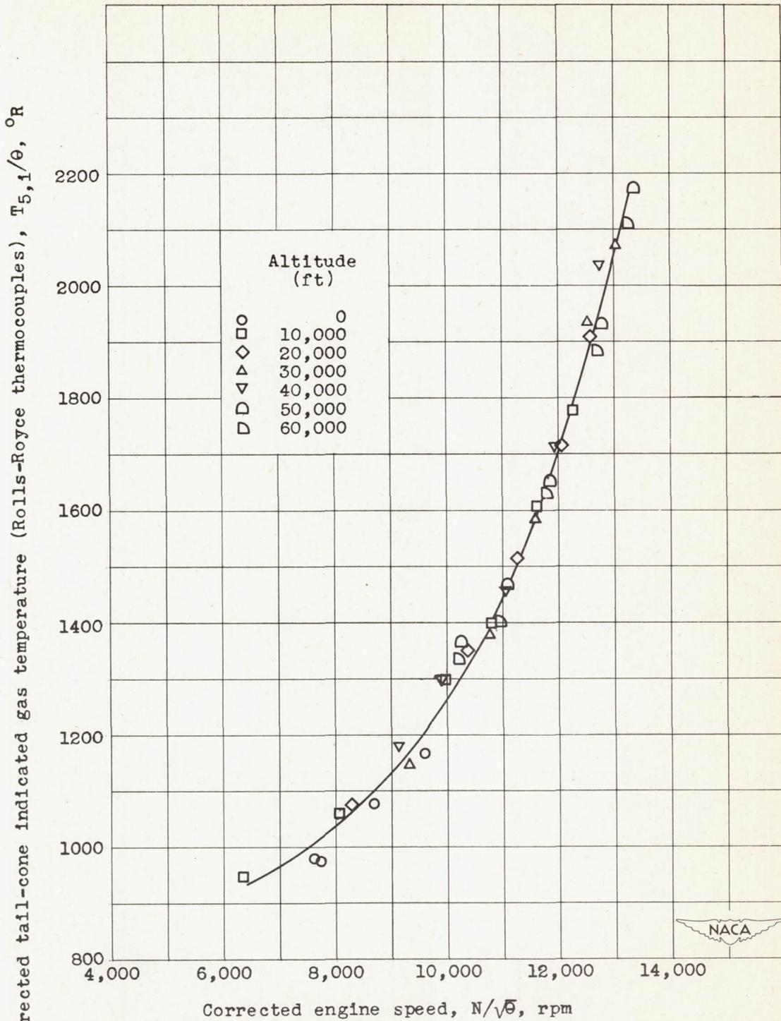
Figure 21. - Concluded. Effect of altitude on corrected indicated gas temperatures. Ram-pressure ratio, 1.30.
