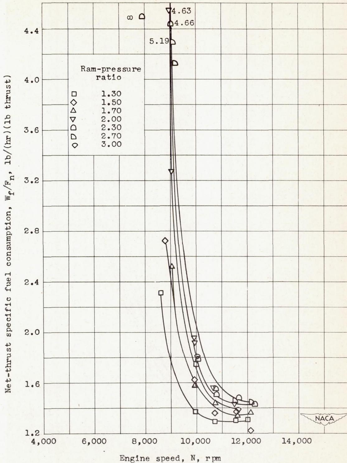
Figure 14. - Effect of ram-pressure ratio on net-thrust specific fuel consumption. Altitude, 30,000 feet.
