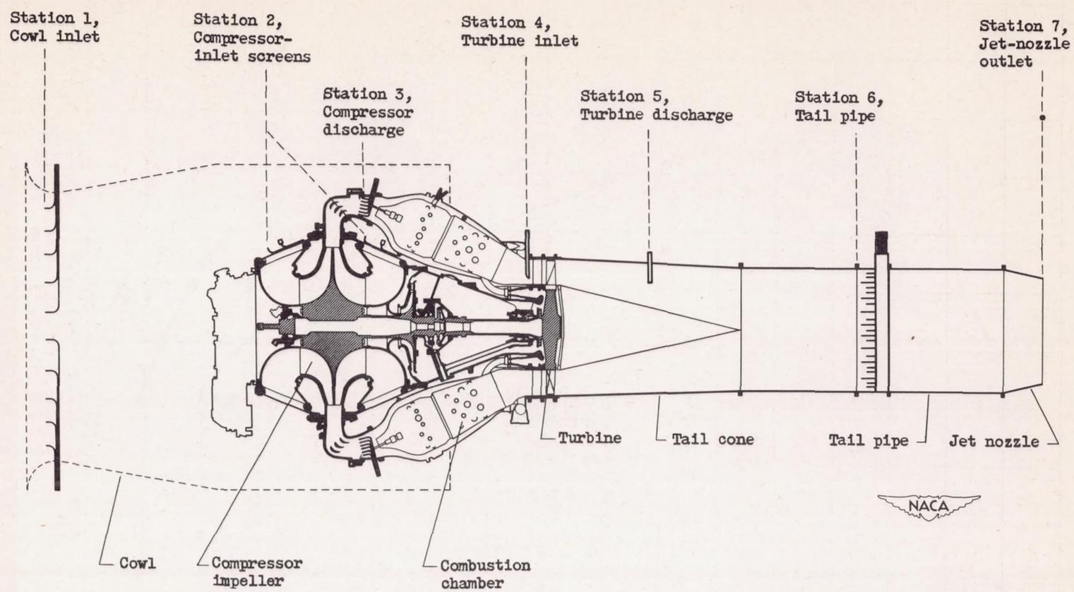
Figure 3. - Sectional side view of British Rolls-Royce Nene II engine showing instrumentation stations.
