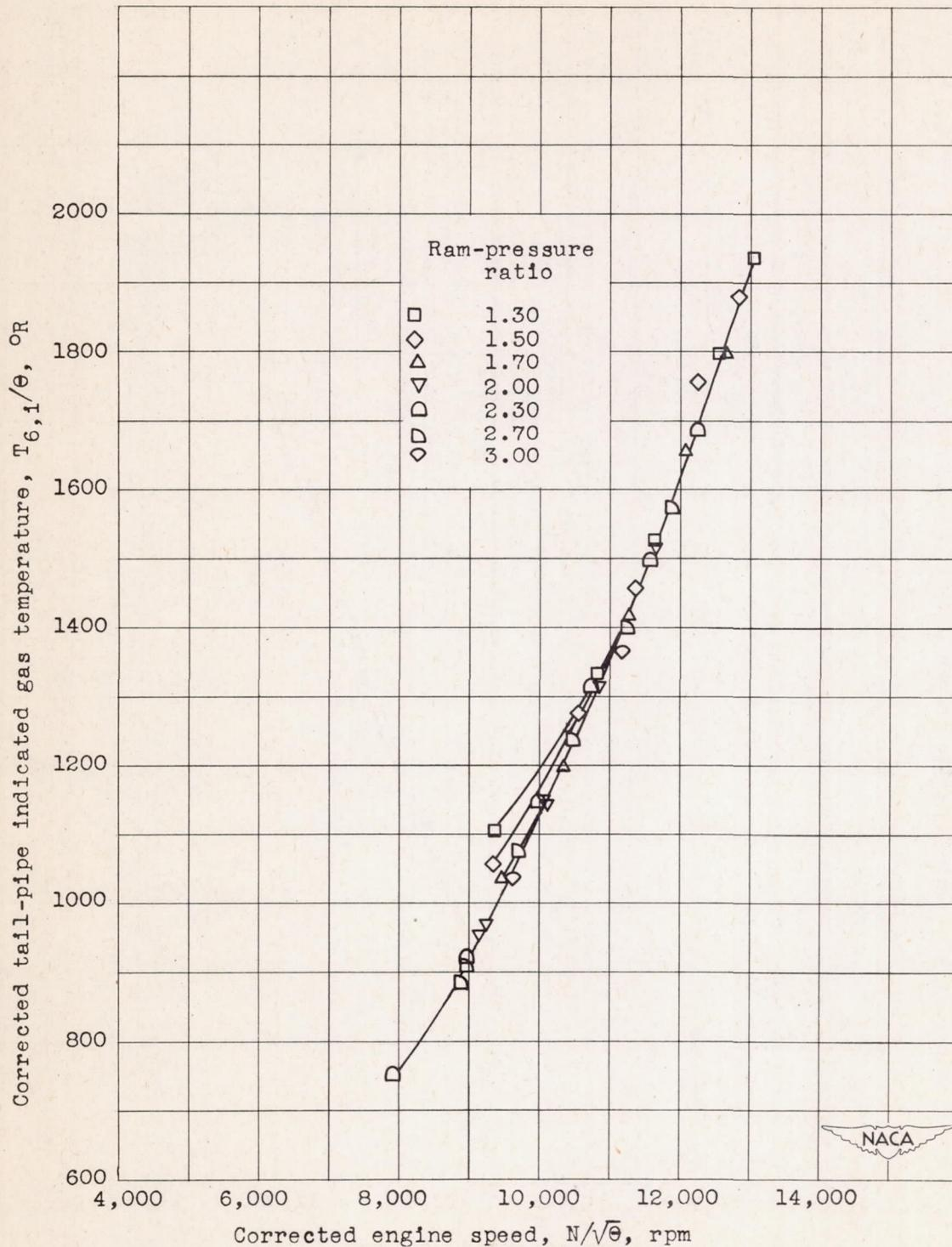
Figure 27. - Effect of ram-pressure ratio on corrected tail-pipe indicated gas temperature. Altitude, 30,000 feet.
