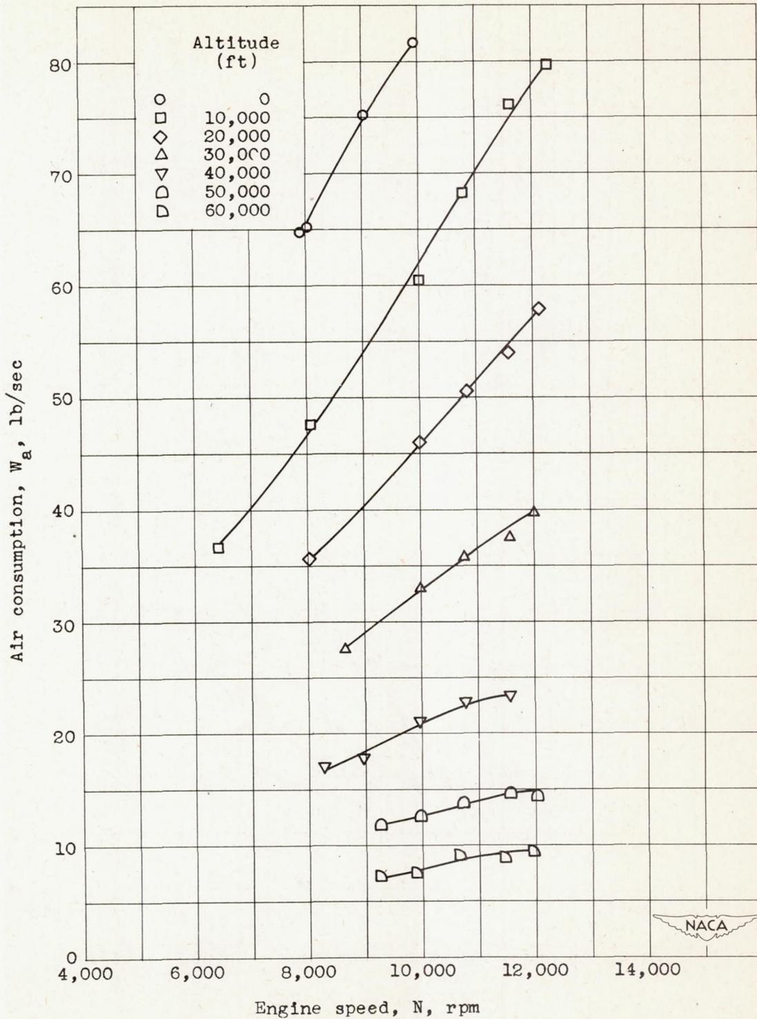
Figure 6. - Effect of altitude on air consumption. Ram-pressure ratio, 1.30.
