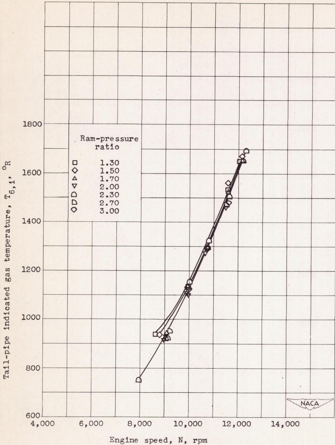
Figure 15. - Effect of ram-pressure ratio on tail-pipe indicated gas temperature. Altitude, 30,000 feet.
