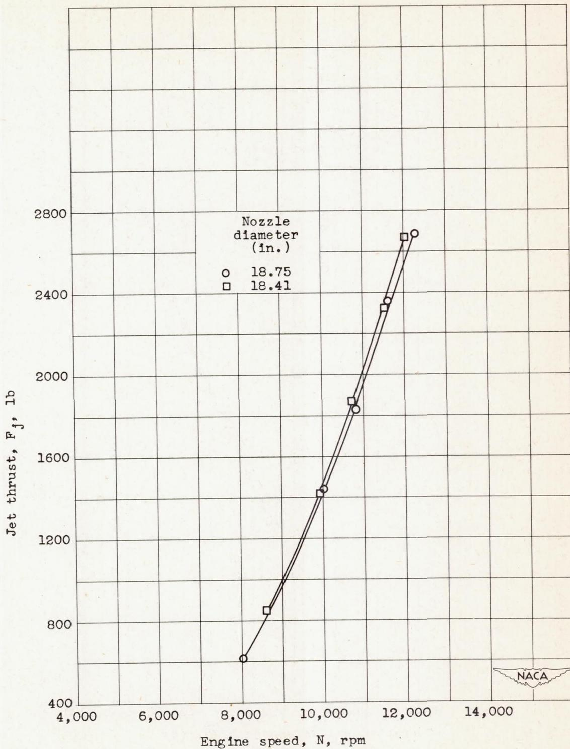
Figure 28. - Effect of jet-nozzle size on jet thrust. Altitude, 30,000 feet; ram-pressure ratio, 1.30.
