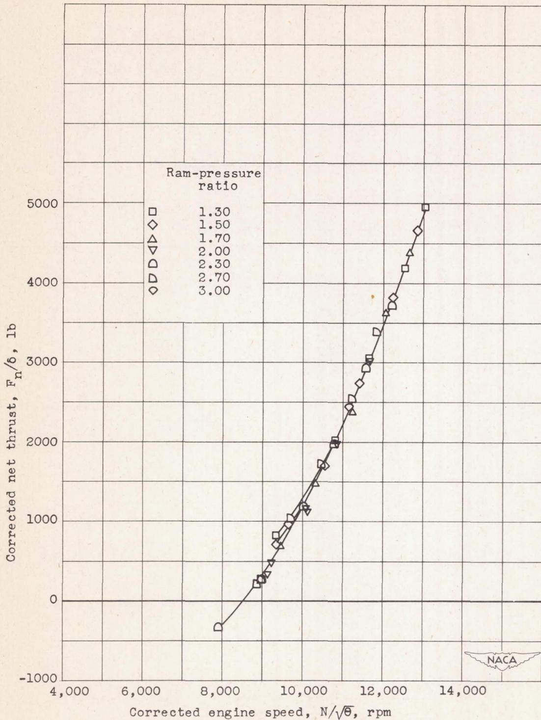
Figure 23. - Effect of ram-pressure ratio on corrected net thrust. Altitude, 30,000 feet.
