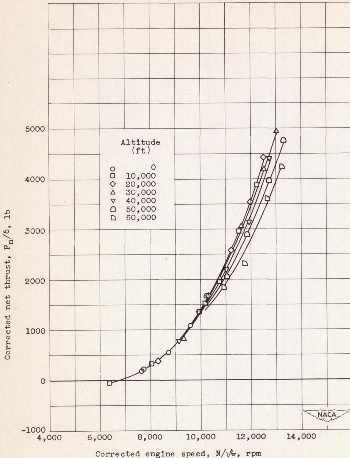
Figure 17. - Effect of altitude on corrected net thrust.
