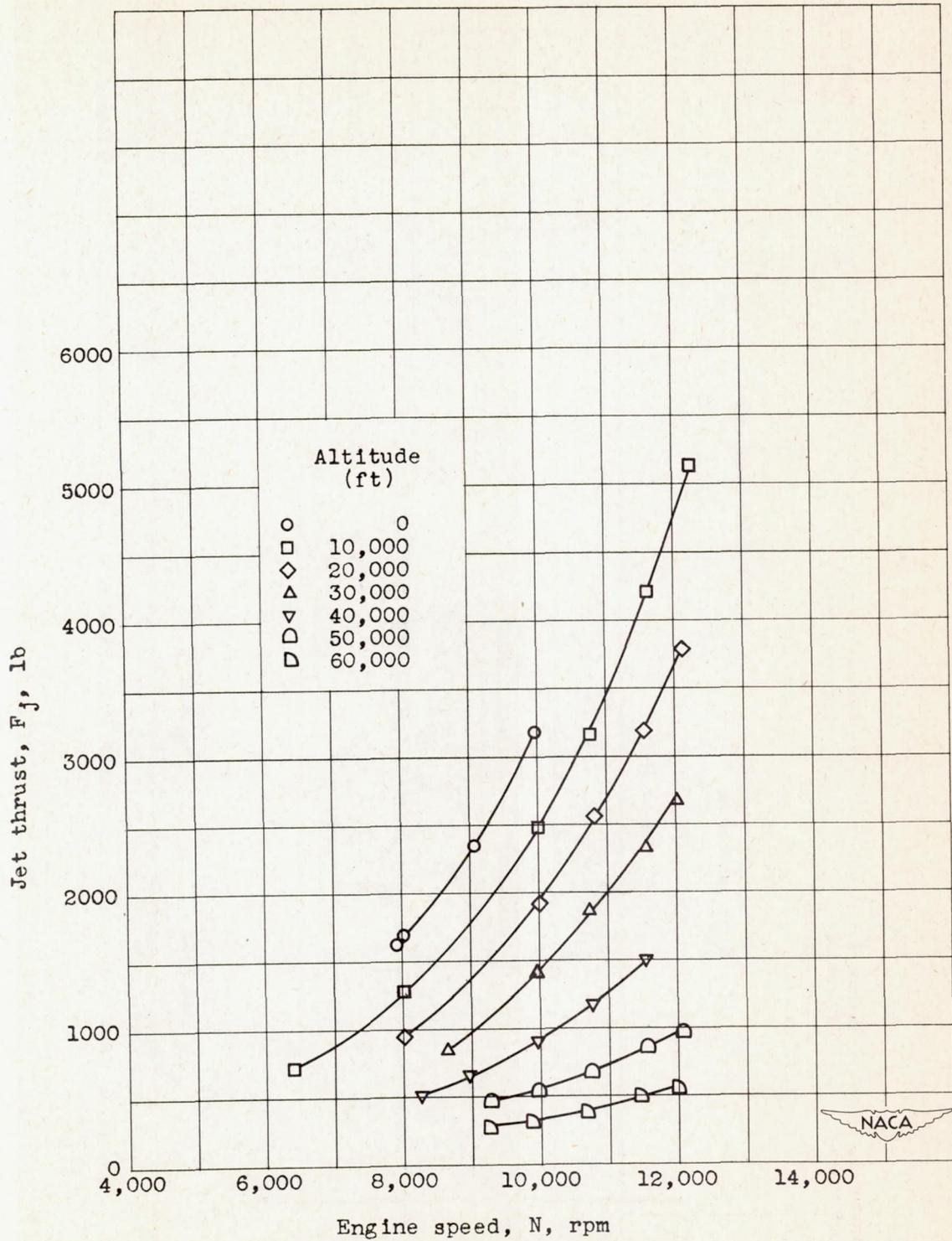
Figure 4. - Effect of altitude on jet thrust. Ram-pressure ratio, 1.30.
