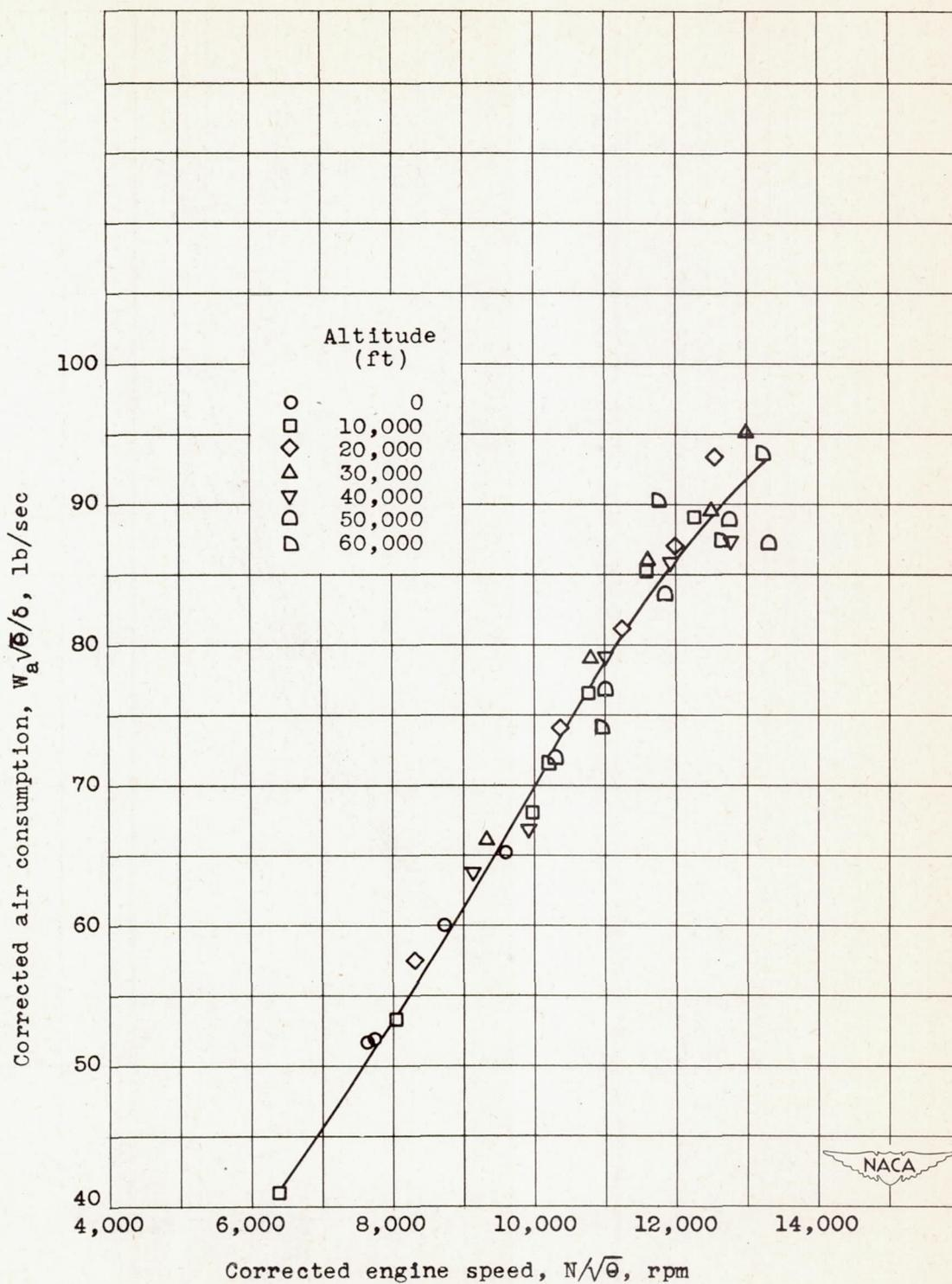
Figure 18. - Effect of altitude on corrected air consumption.
