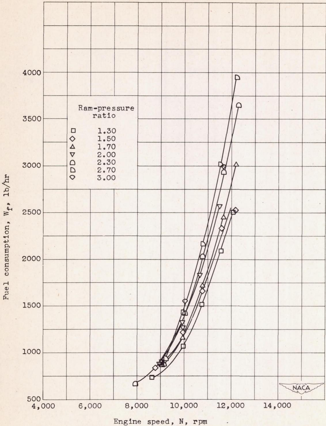
Figure 13. - Effect of ram-pressure ratio on fuel consumption. Altitude, 30,000 feet.
