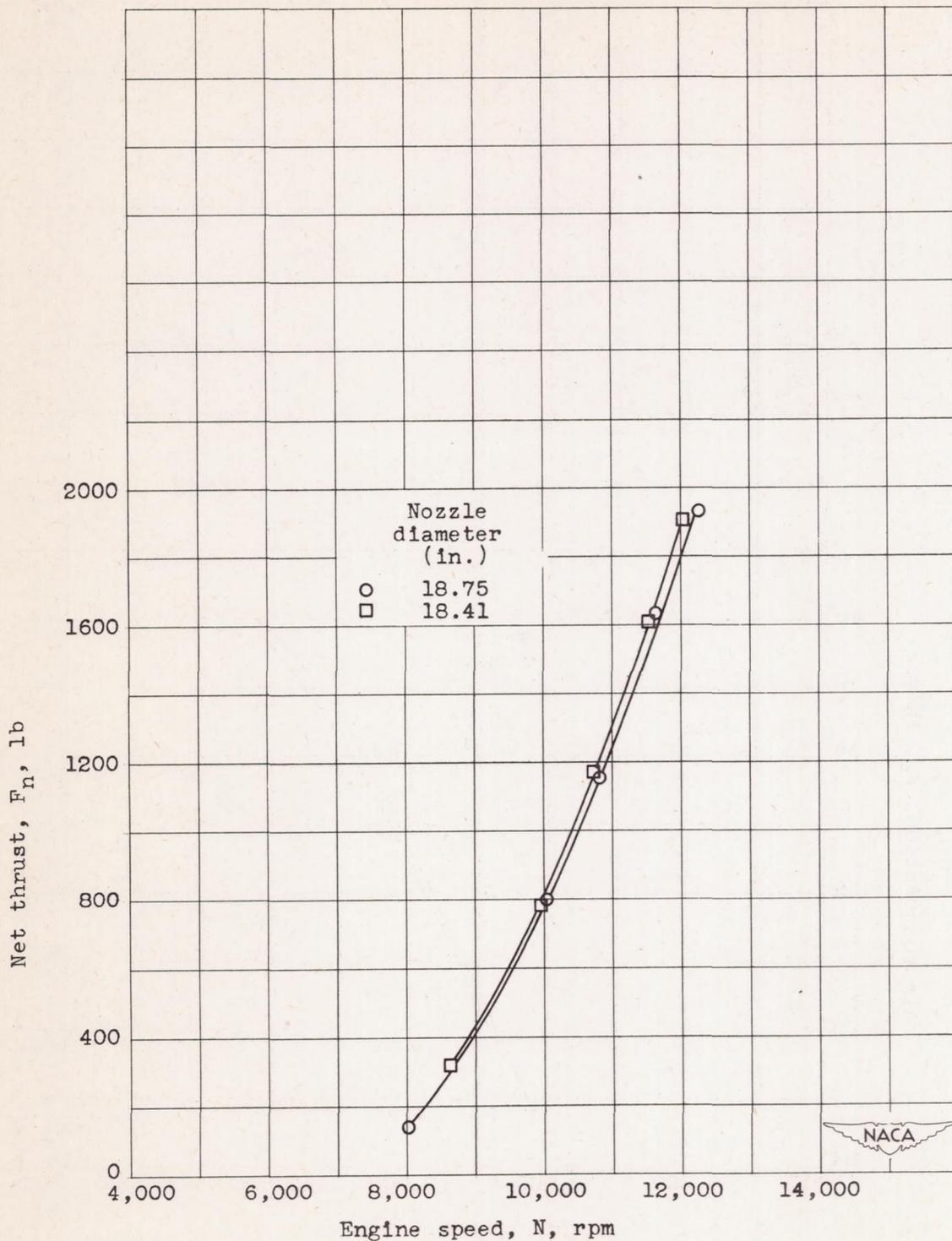
Figure 29. - Effect of jet-nozzle size on net thrust. Altitude, 30,000 feet; ram-pressure ratio, 1.30.
