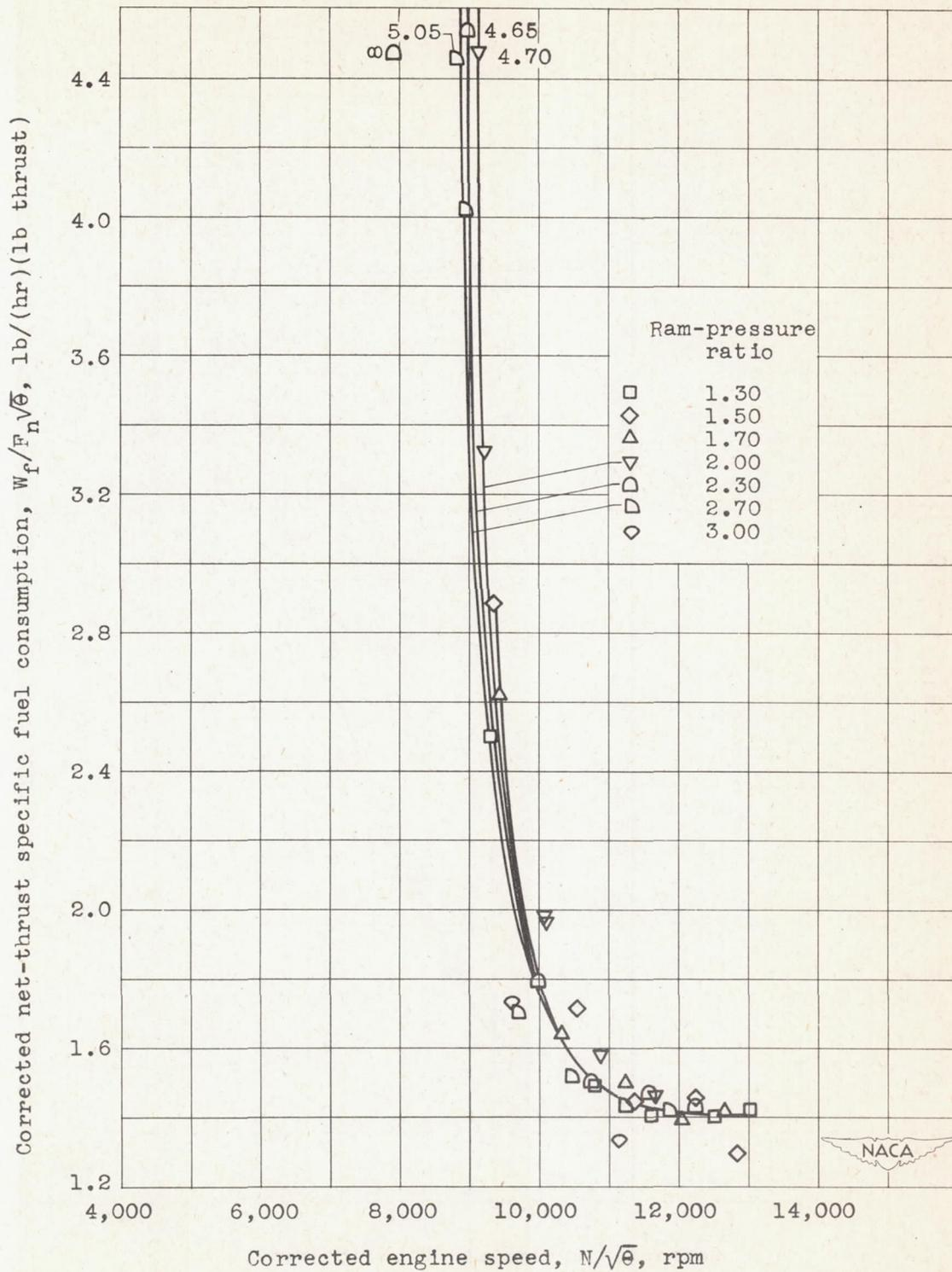
Figure 26. - Effect of ram-pressure ratio on corrected net-thrust specific fuel consumption. Altitude, 30,000 feet.
