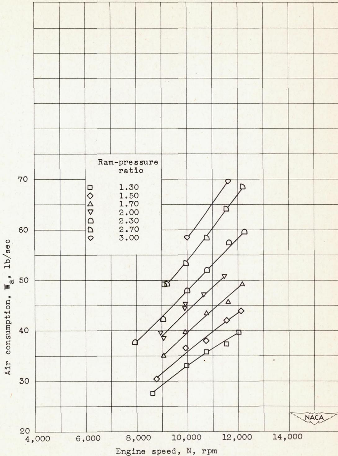
Figure 12. - Effect of ram-pressure ratio on air consumption.
