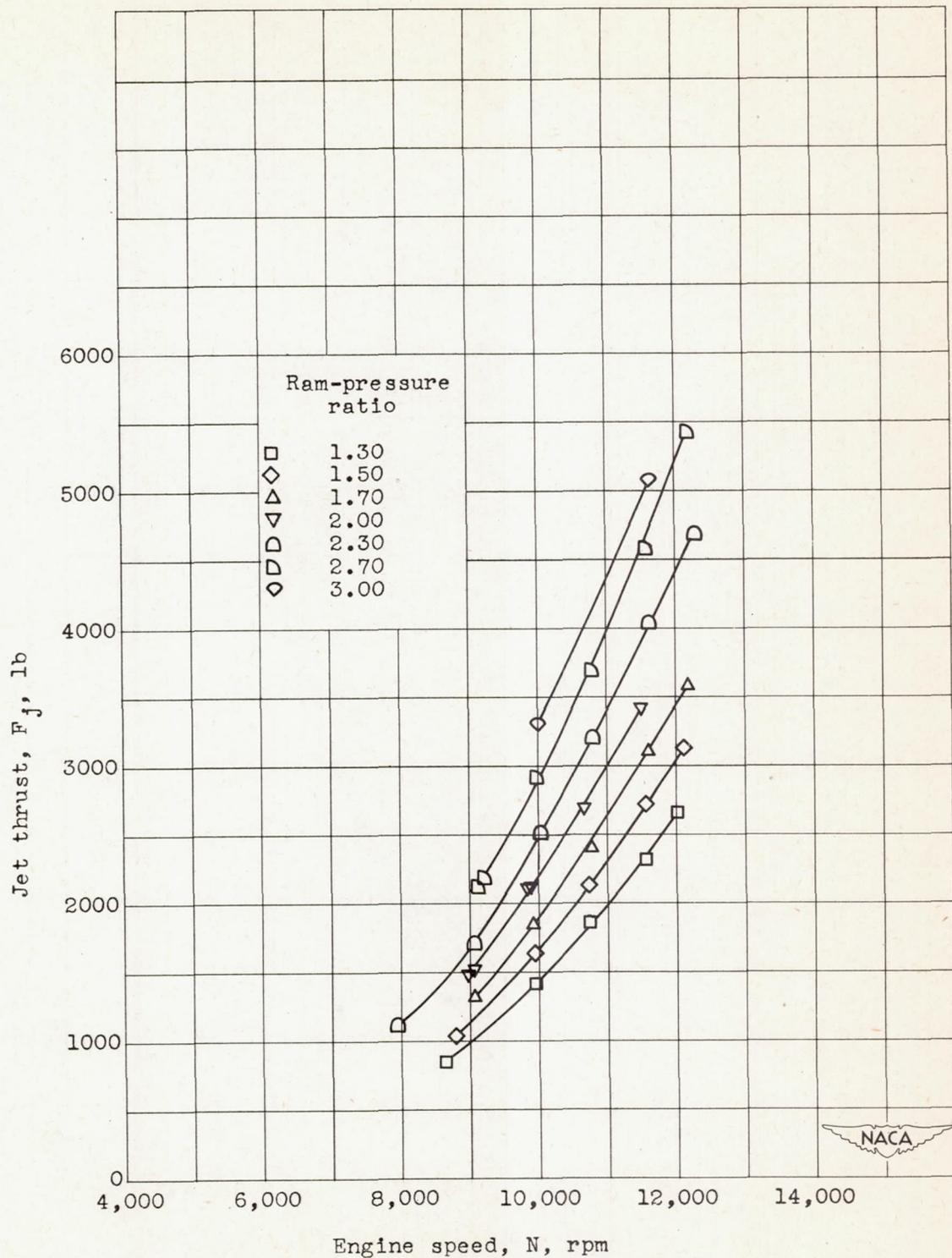
Figure 10. - Effect of ram-pressure ratio on jet thrust.
