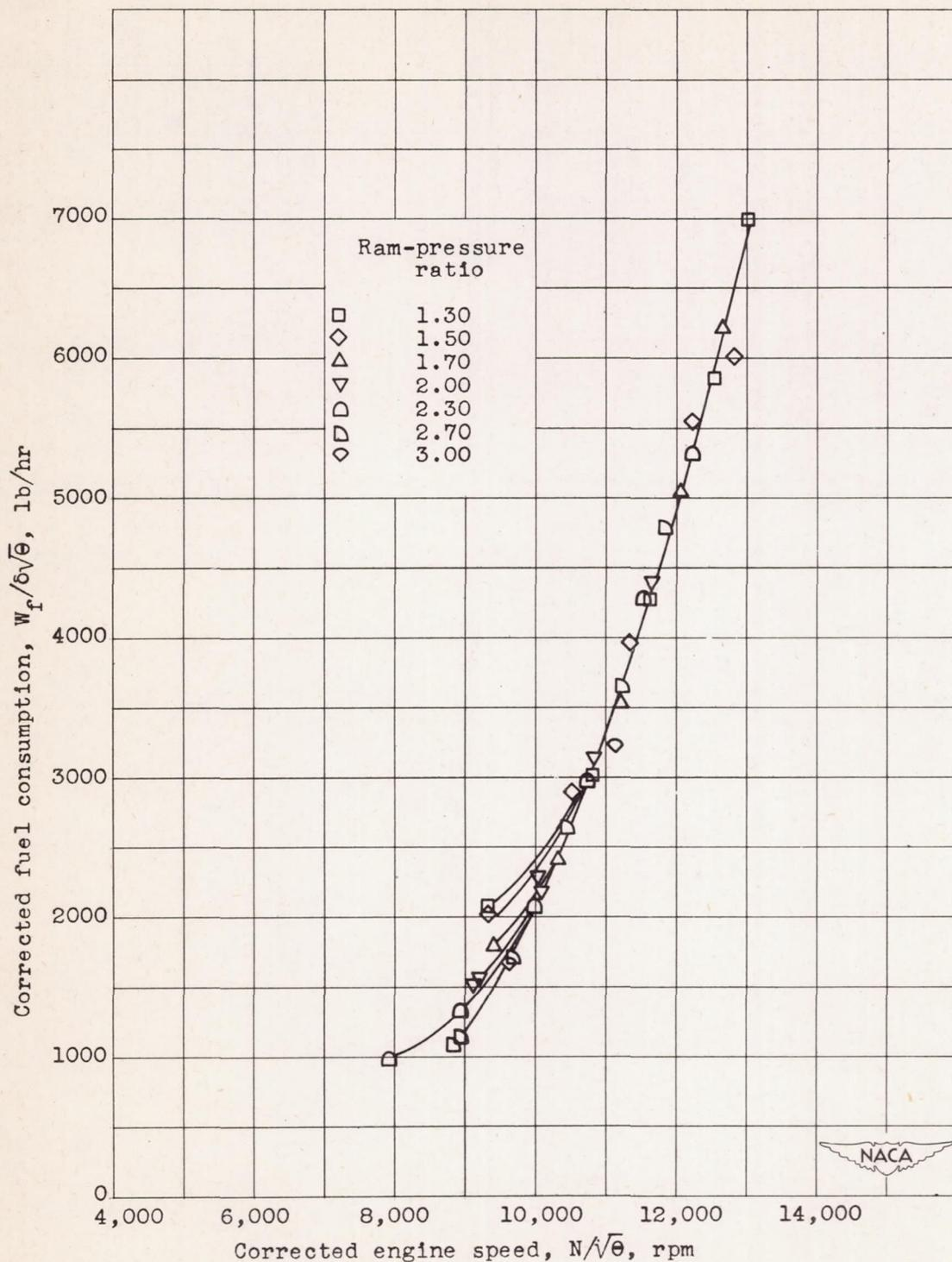
Figure 25. - Effect of ram-pressure ratio on corrected fuel consumption. Altitude, 30,000 feet.
