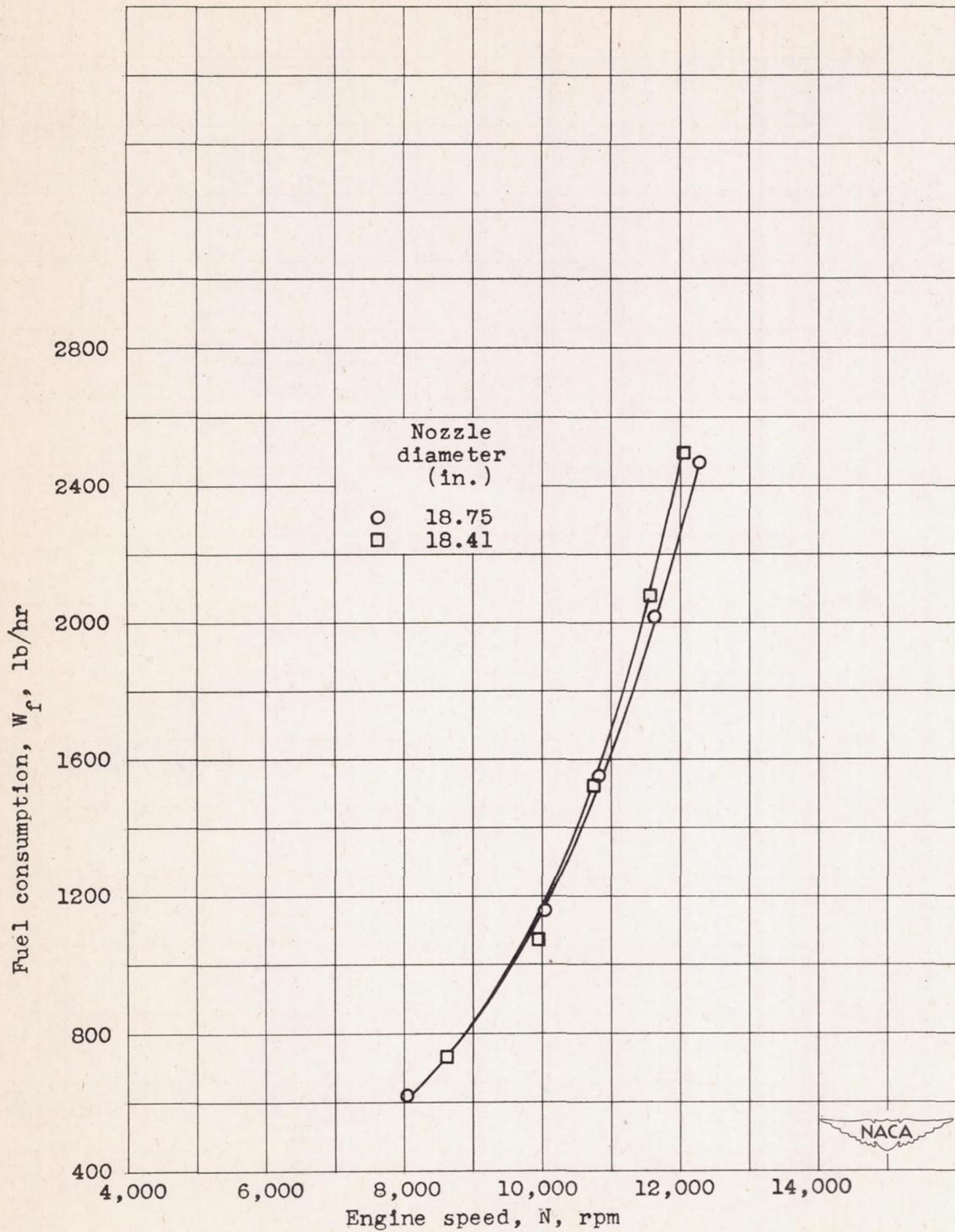
Figure 31. - Effect of jet-nozzle size on fuel consumption.
