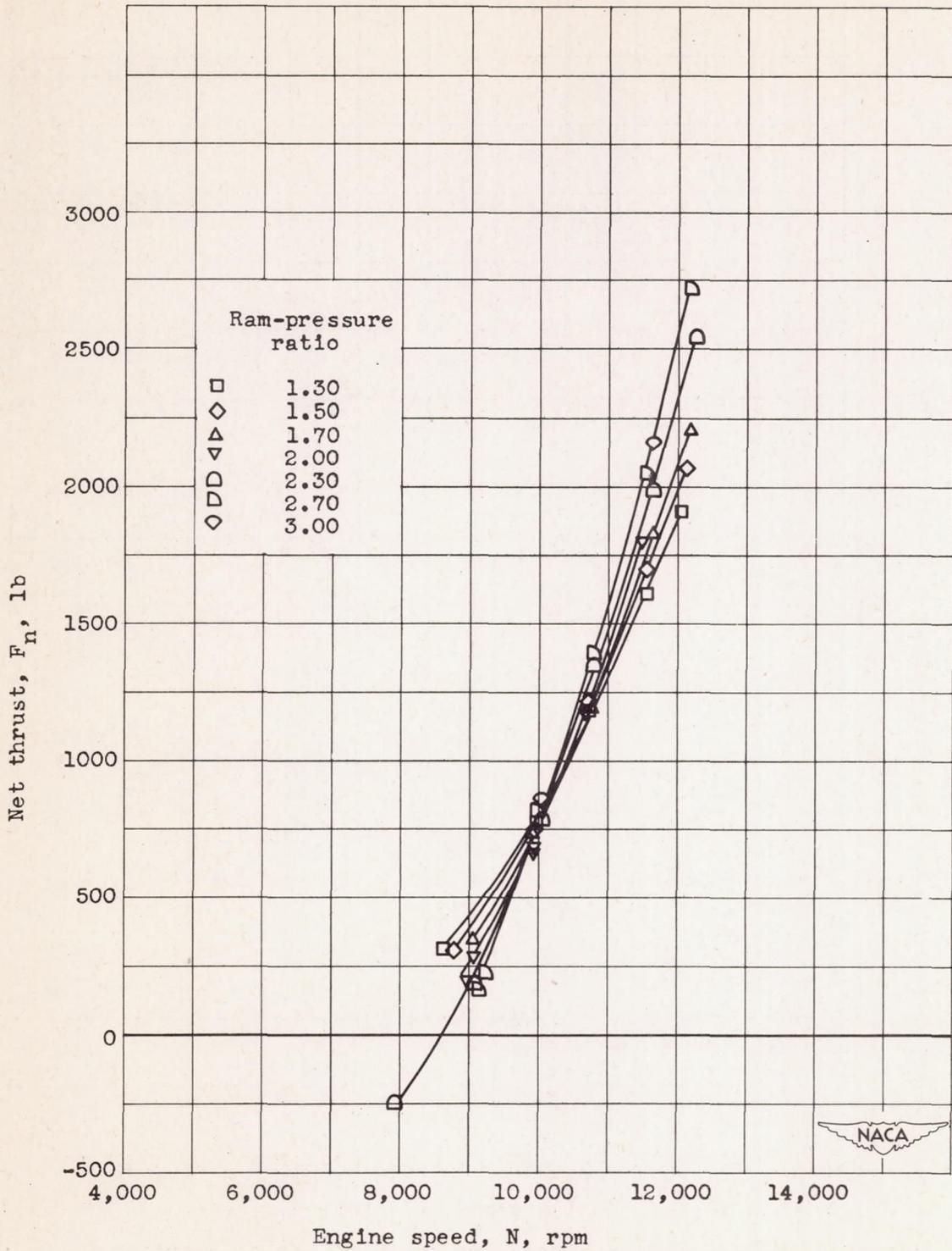
Figure 11. - Effect of ram-pressure ratio on net thrust.
