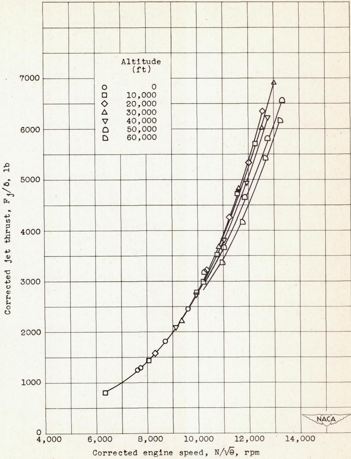
Figure 16. - Effect of altitude on corrected jet thrust.
