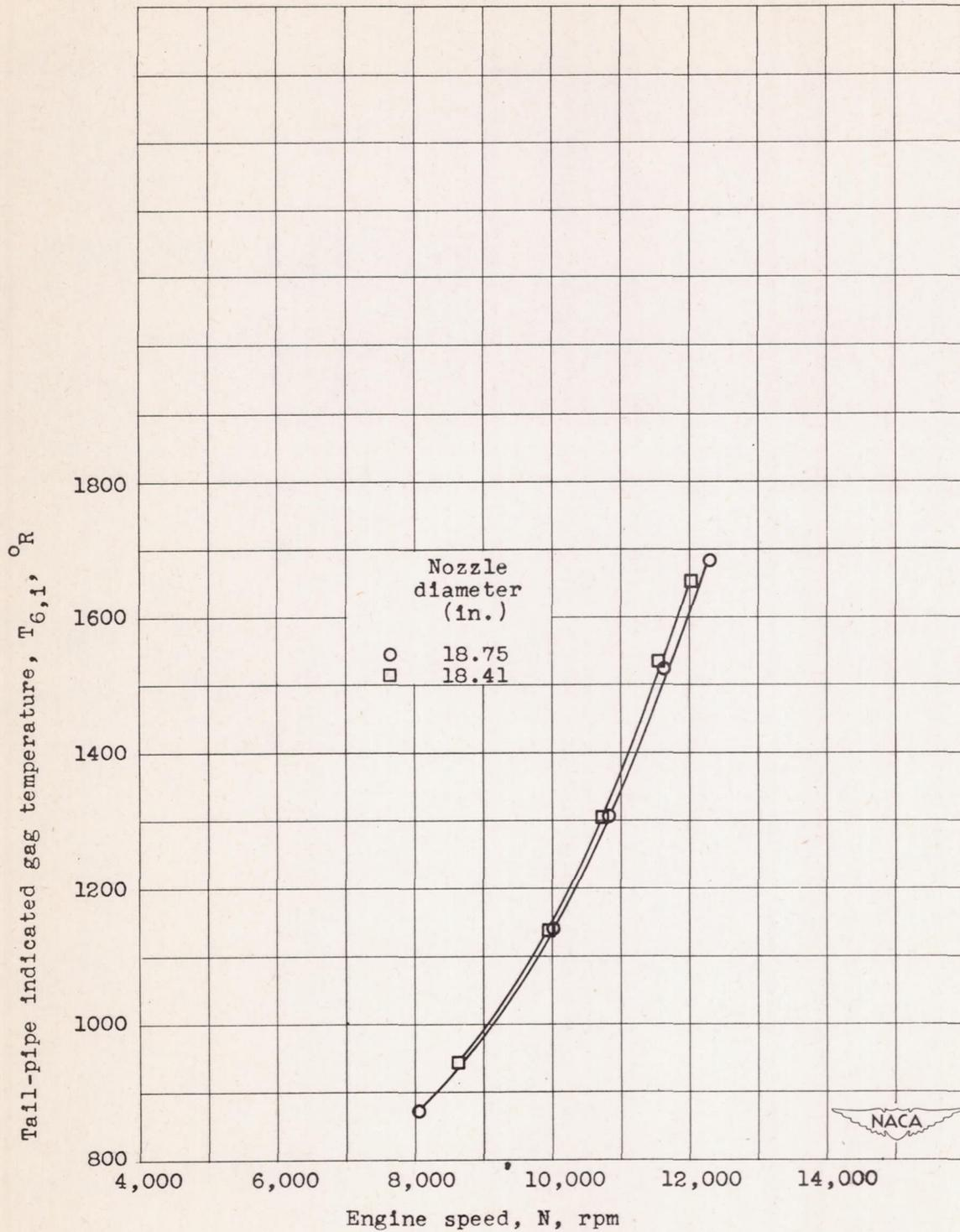
Figure 33. - Effect of jet-nozzle size on tail-pipe indicated gas temperature. Altitude, 30,000 feet; ram-pressure ratio, 1.30.
