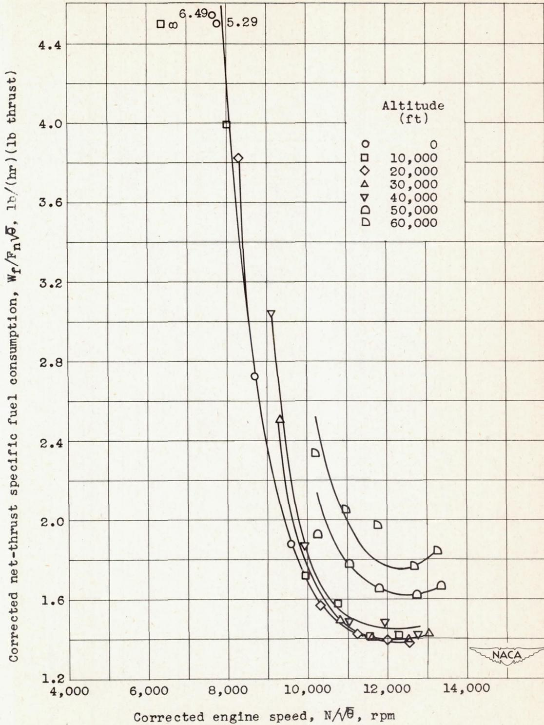
Figure 20. - Effect of altitude on corrected net-thrust specific fuel consumption. Ram-pressure ratio, 1.30.
