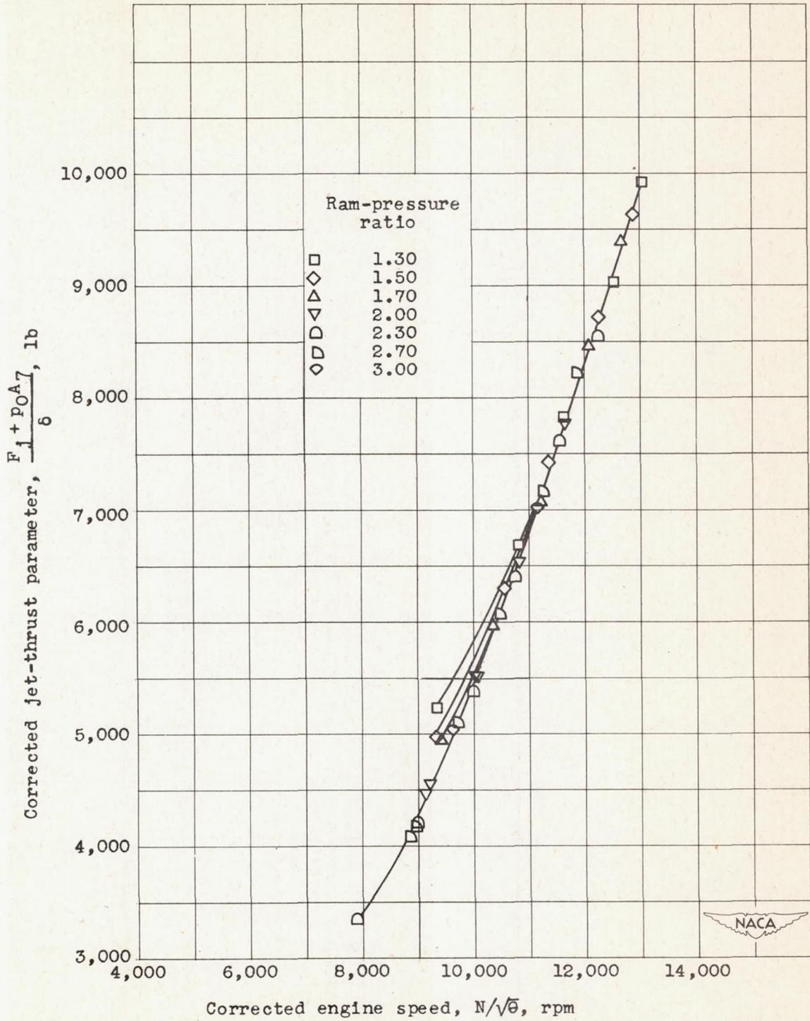
(b) Corrected jet-thrust parameter,  $\frac{F_j + p_0 A_7}{\delta}$
