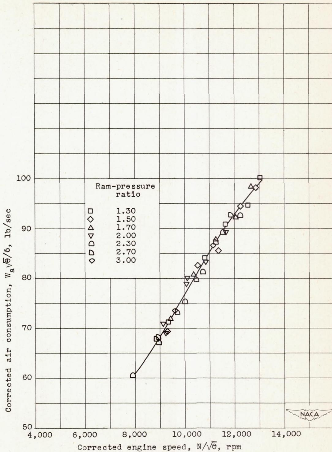
Figure 24. - Effect of ram-pressure ratio on corrected air consumption. Altitude, 30,000 feet.
