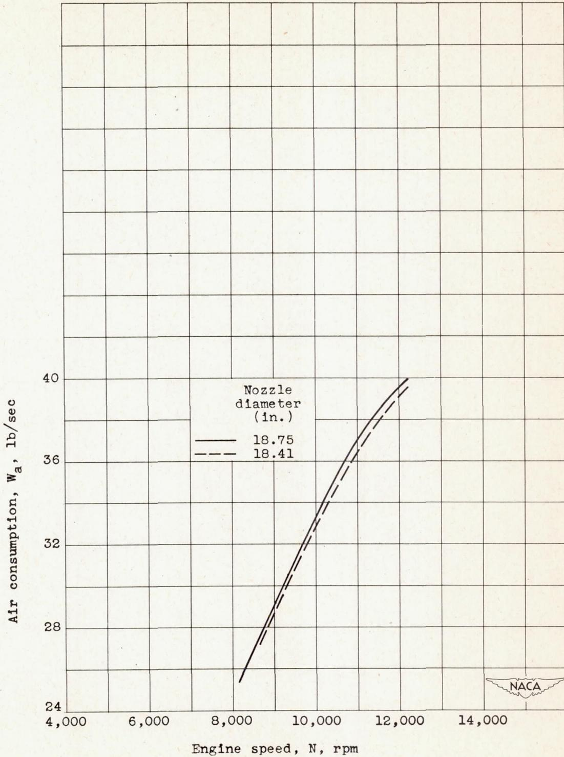
Figure 30. - Effect of jet-nozzle size on air consumption.
