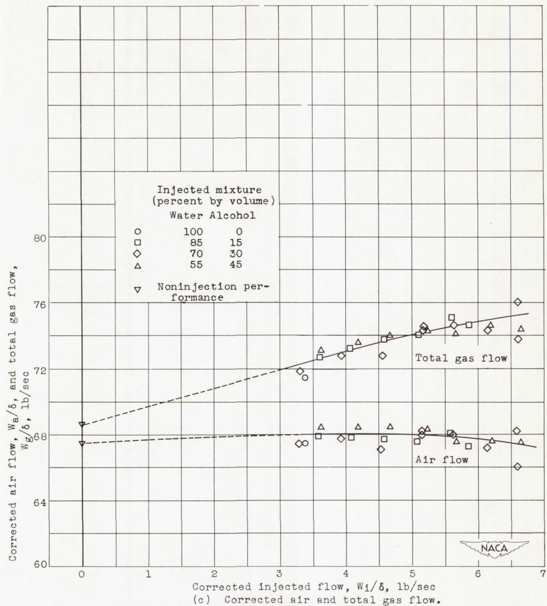
Figure 7. - Continued. Turbojet-engine performance with three-stage system of water-alcohol injection investigated at sea-level, zero-ram conditions. Data corrected to engine inlet-air temperature of  $80^{\circ}$  F; engine speed, 7610 rpm; exhaust-gas temperature,  $1200^{\circ}$  F.
