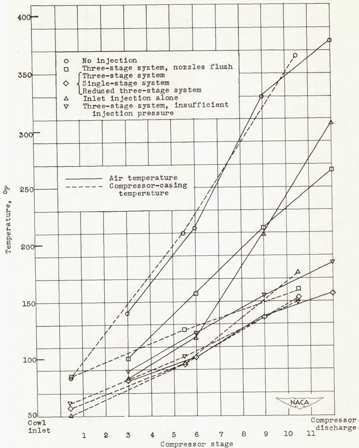
(c) Longitudinal temperature distribution along compressor.
