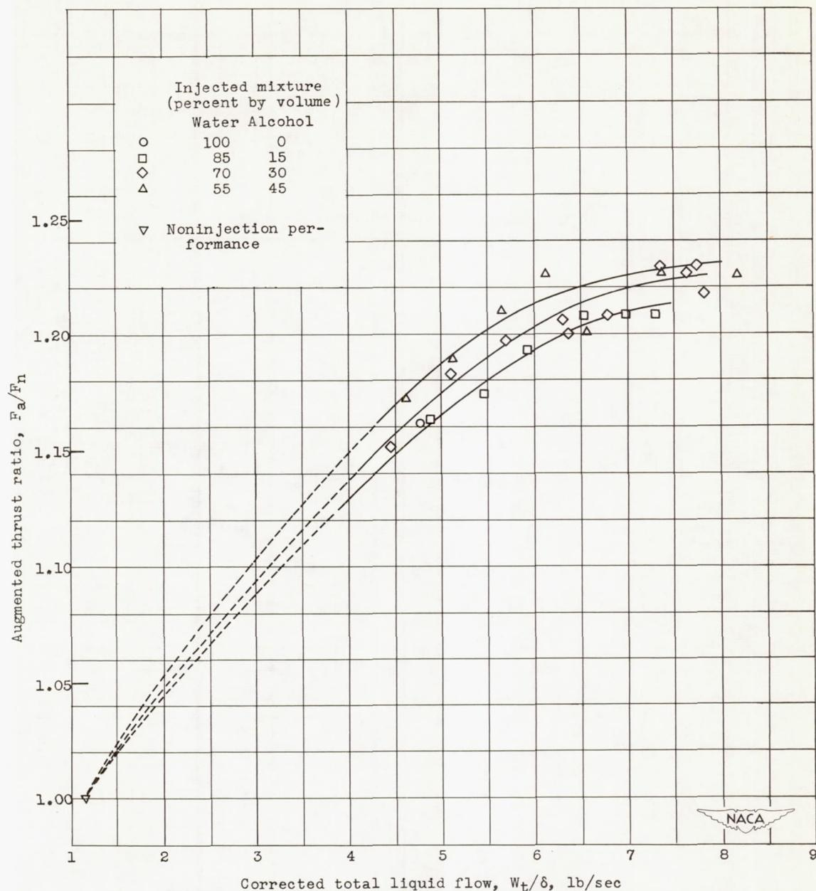
Figure 8. - Variation of augmented thrust ratio with corrected total liquid flow for three-stage system of water-alcohol injection investigated at sea-level, zero-ram conditions. Data corrected to an engine inlet-air temperature of 80° F; engine speed, 7610 rpm; exhaust gas temperature, 1200° F.
