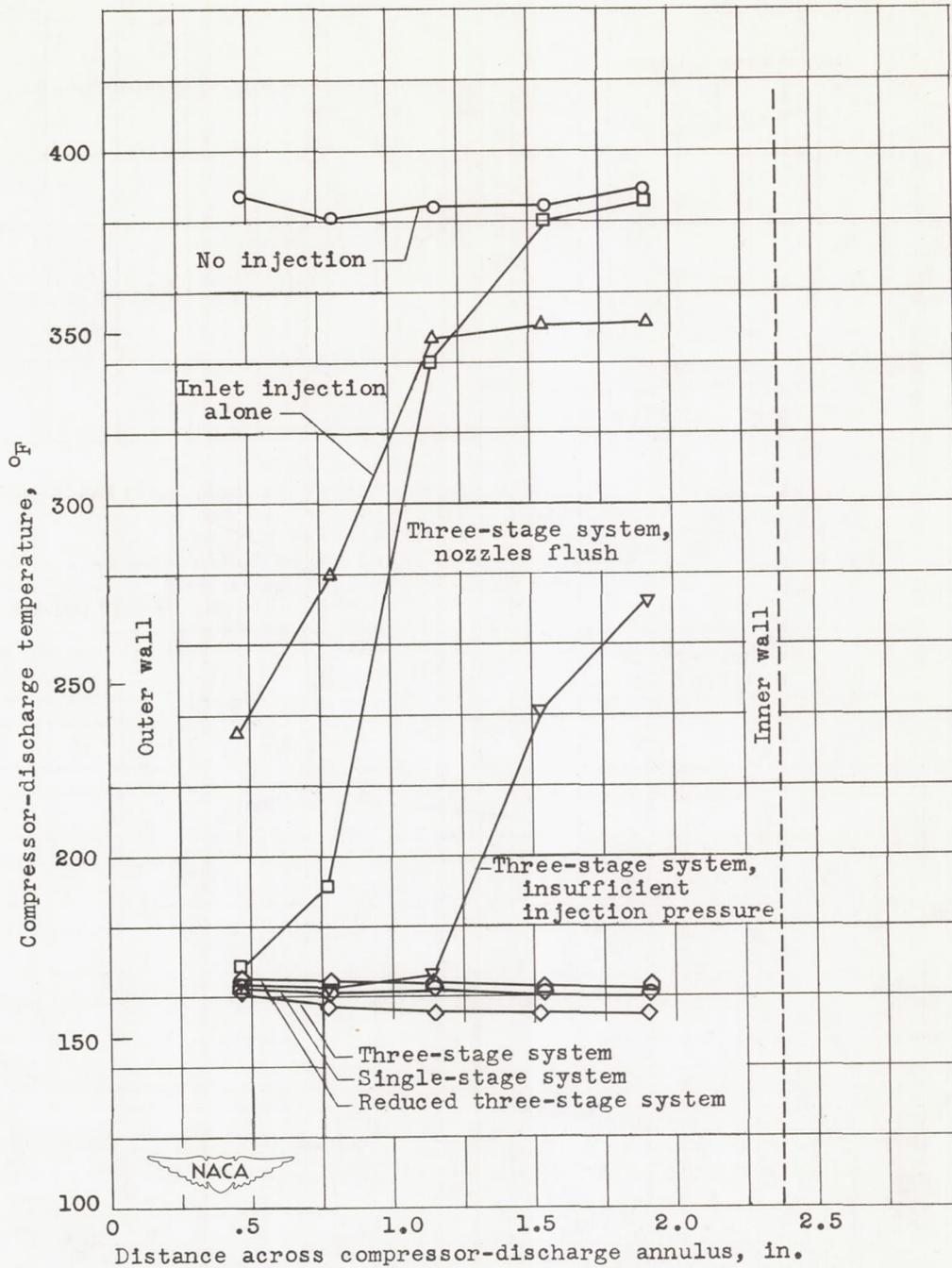
(a) Radial temperature distribution across compressor-discharge annulus.
