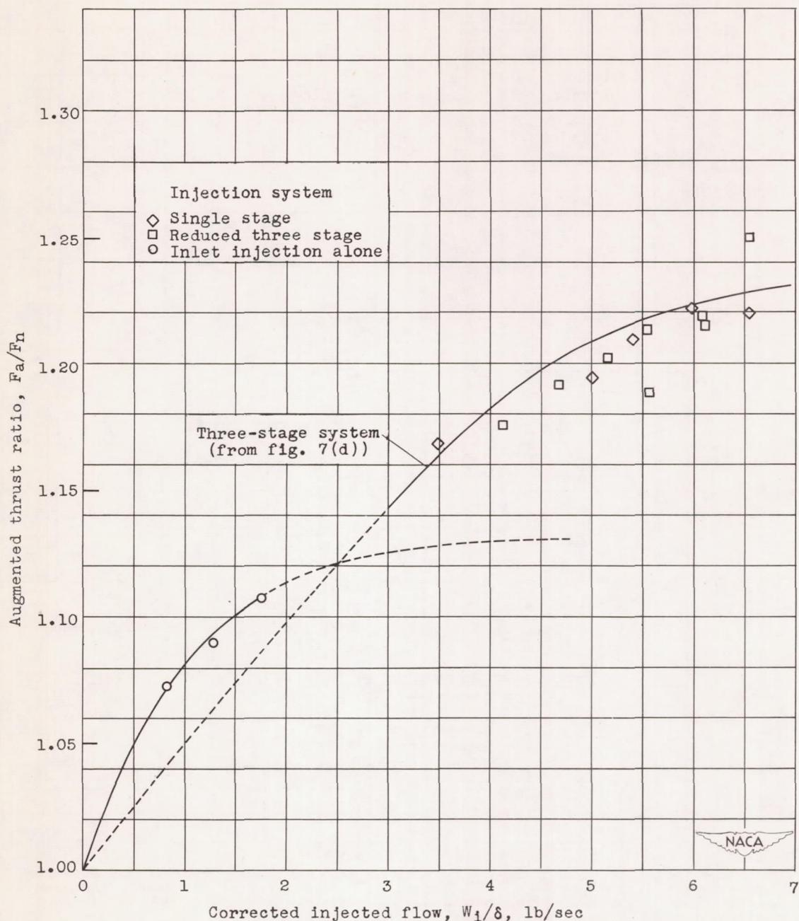
Figure 9. - Augmented performance of turbojet engine with several injection systems investigated at sea-level, zero-ram conditions. Data corrected to engine inlet-air temperature,  $80^{\circ}$  F; engine speed, 7610 rpm; exhaust-gas temperature,  $1200^{\circ}$  F.
