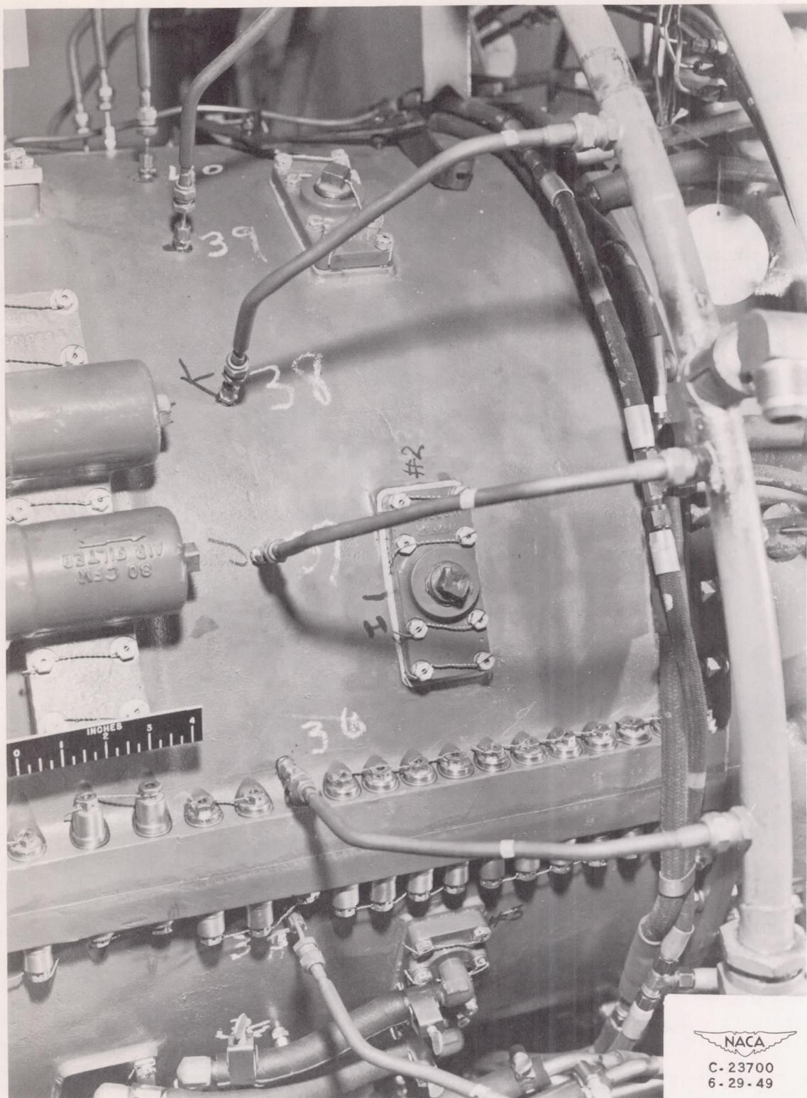
Figure 4. - Interstage-nozzle extension tubes of single-stage system installed in sixth stage of compressor. Extension tubes are shown connected to injection manifold.
