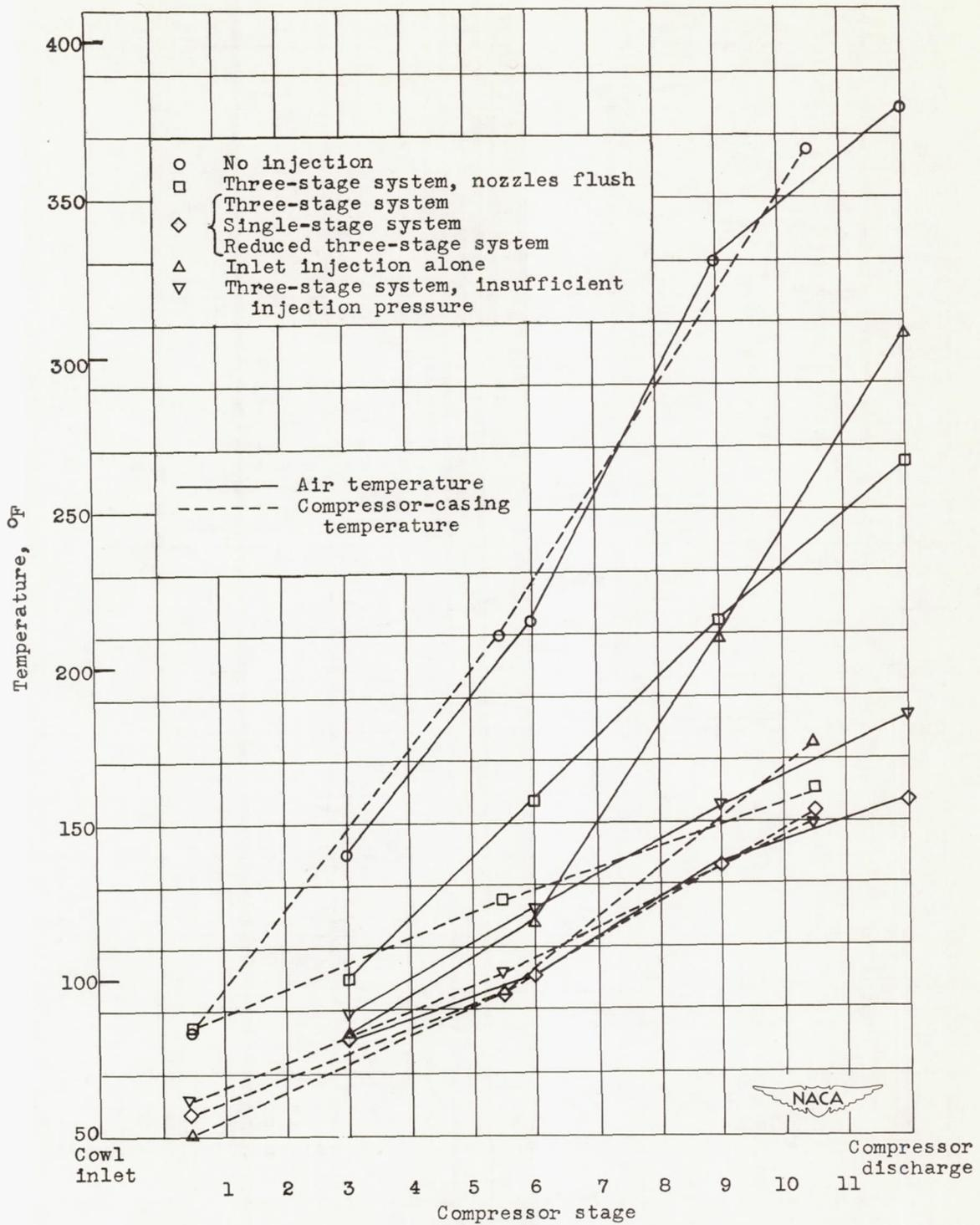
(c) Longitudinal temperature distribution along compressor.
