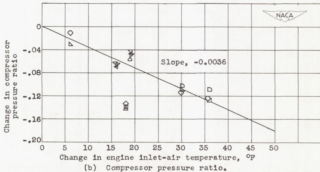
Figure 6. - Experimentally determined variation of augmented turbojet-engine performance resulting from changes in engine inlet-air temperature.
