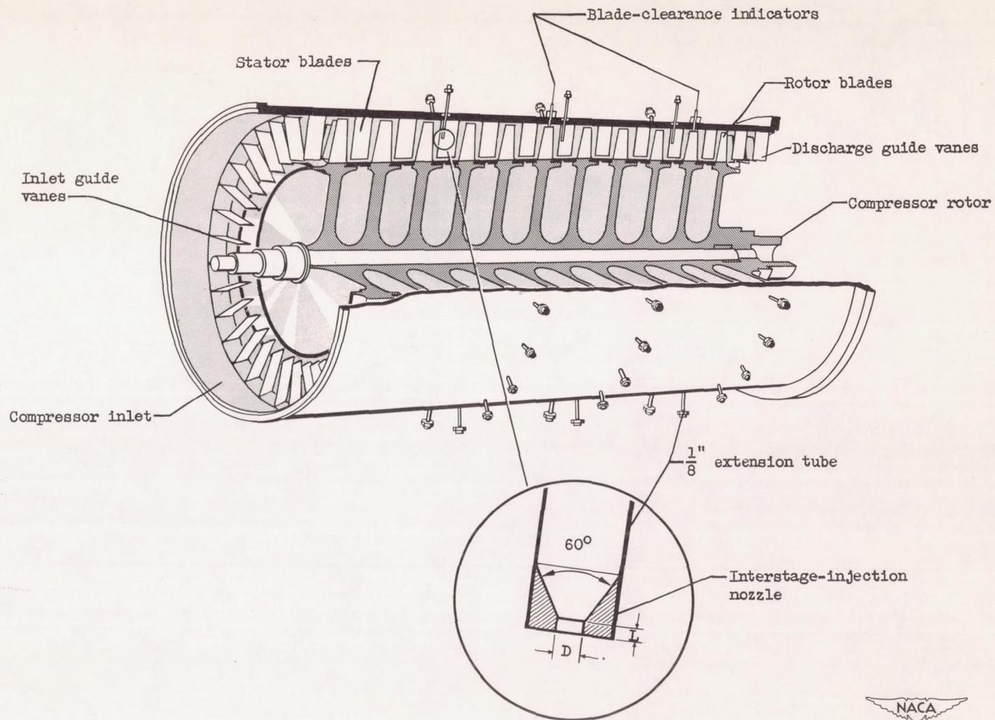
Figure 3. - Diagrammatic sketch of installation of interstage-injection nozzles in axial-flow compressor.
