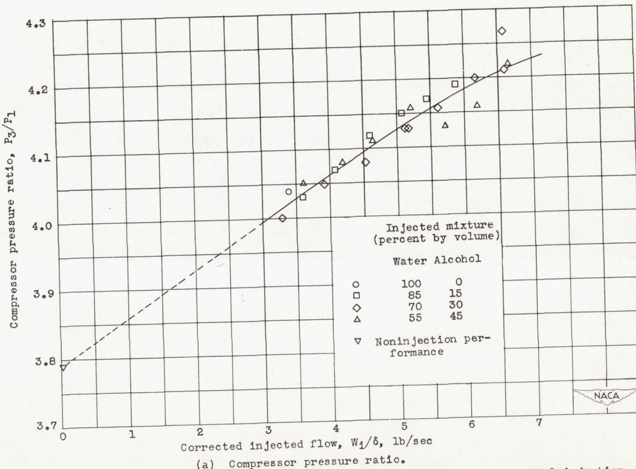
Figure 7. - Turbojet-engine performance with three-stage system of water-alcohol injection investigated at sea-level, zero-ram conditions. Data corrected to engine inlet-air temperature of 80° F; engine speed, 7610 rpm; exhaust-gas temperature, 1200° F.
