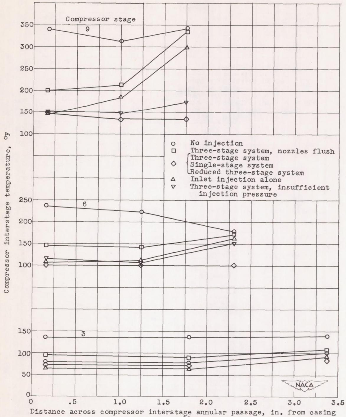
(b) Radial temperature distribution across compressor interstage annular passage.
