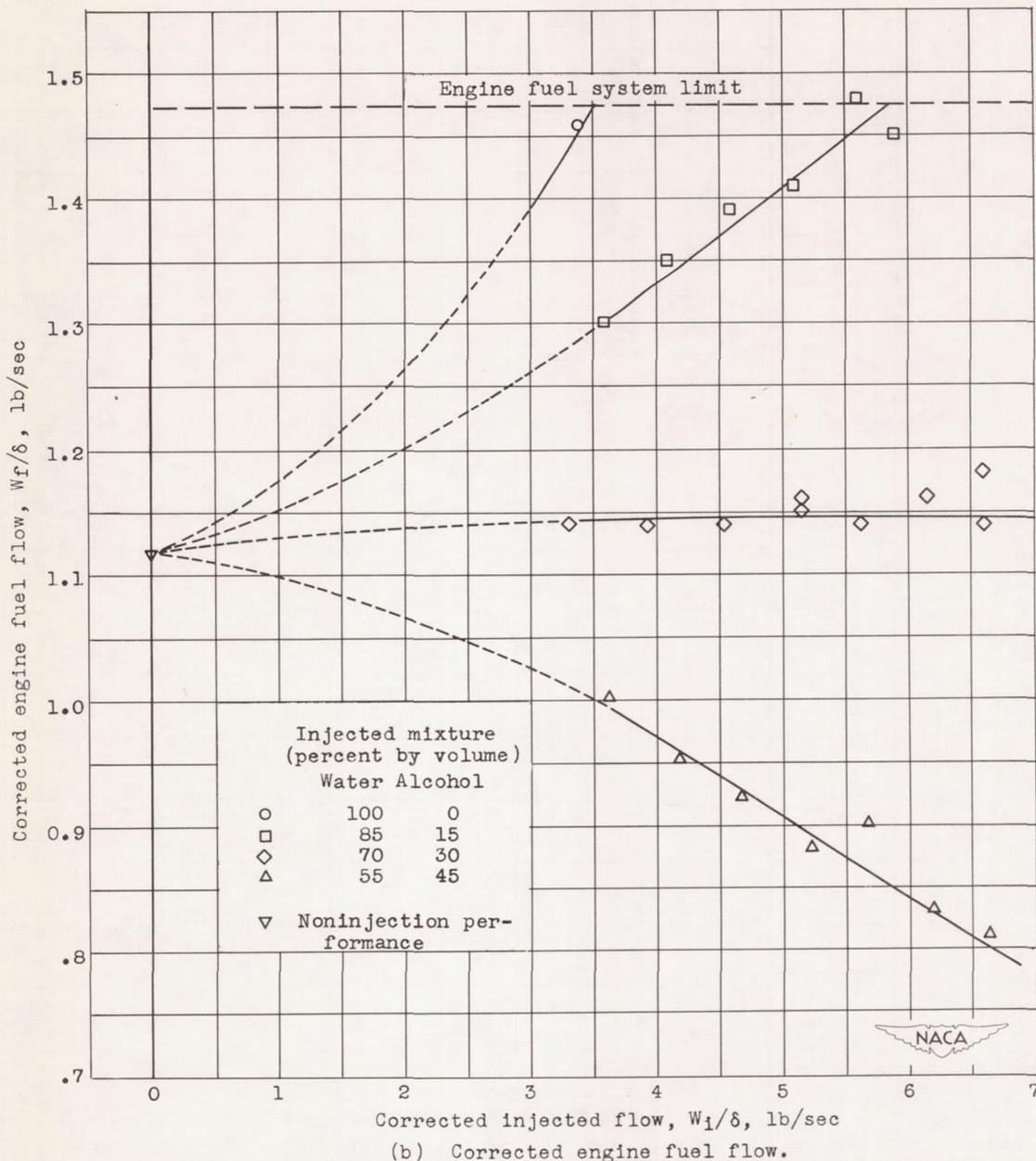
Figure 7. - Continued. Turbojet-engine performance with three-stage system of water-alcohol injection investigated at sea-level, zero-rpm conditions. Data corrected to engine inlet-air temperature of 80° F; engine speed, 7610 rpm; exhaust-gas temperature, 1200° F.
