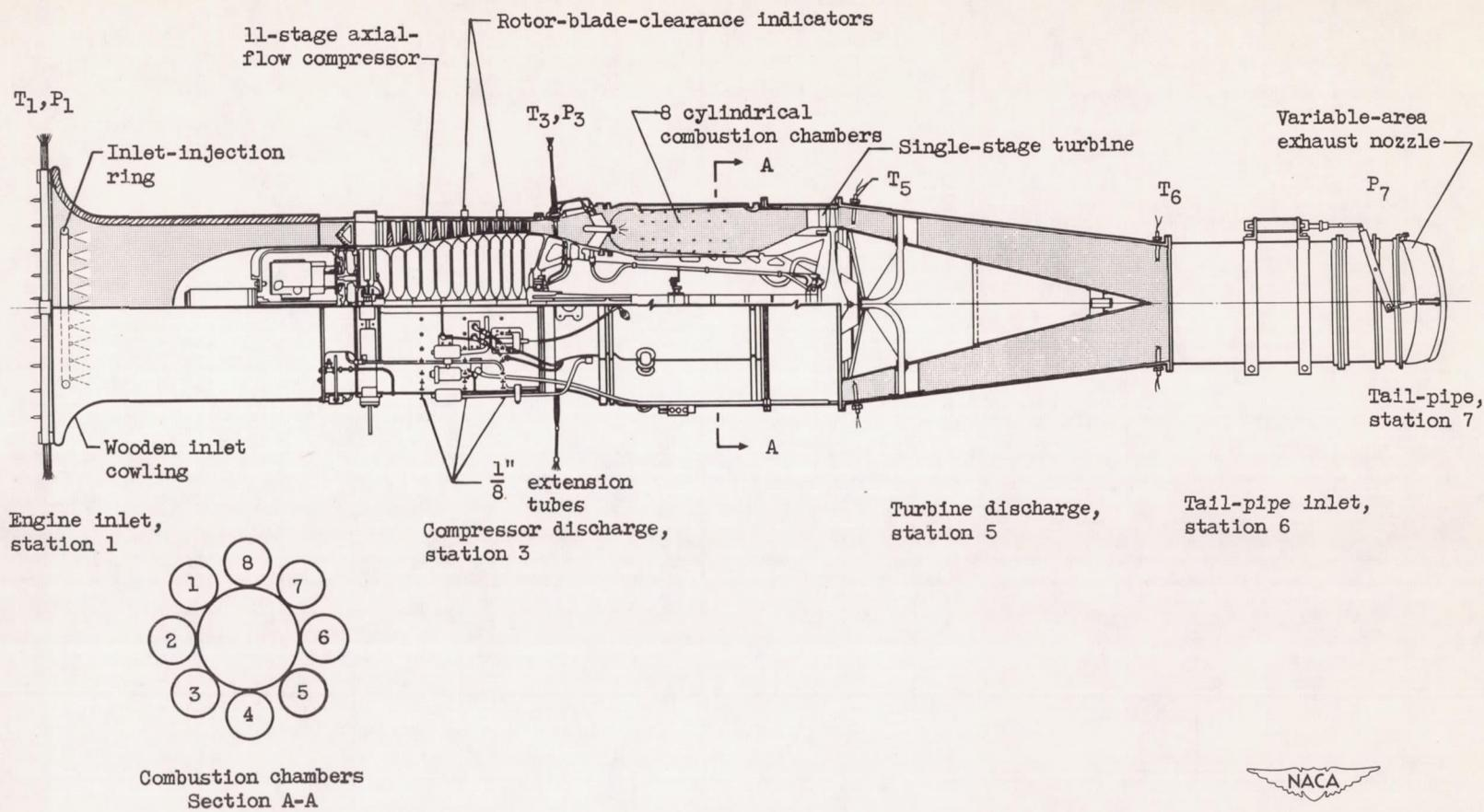
Figure 5. - Engine instrumentation.
