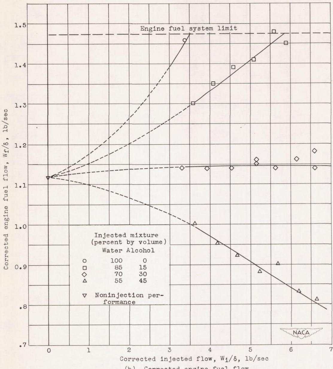
Figure 7. - Continued. Turbojet-engine performance with three-stage system of water-alcohol injection investigated at sea-level, zero-ram conditions. Data corrected to engine inlet-air temperature of 80° F; engine speed, 7610 rpm; exhaust-gas temperature, 1200° F.
