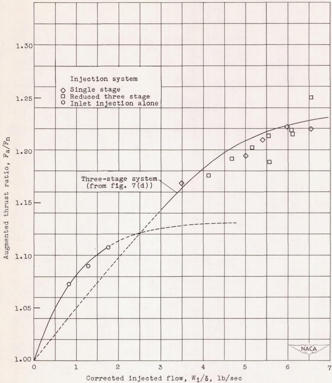
Figure 9. - Augmented performance of turbojet engine with several injection systems investigated at sea-level, zero-ram conditions. Data corrected to engine inlet-air temperature, 80° F; engine speed, 7610 rpm; exhaust-gas temperature, 1200° F.
