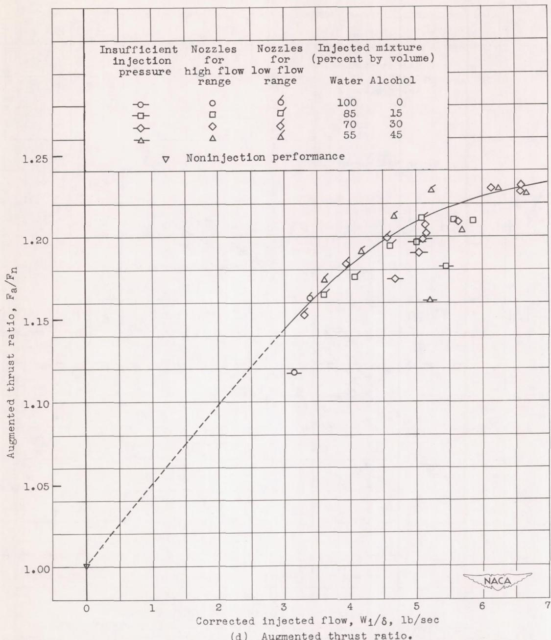
Figure 7. - Concluded. Turbojet-engine performance with three-stage system of water-alcohol injection investigated at sea-level, zero-ram conditions. Data corrected to engine inlet-air temperature of  $800^{\circ}$  F; engine speed, 7610 rpm; exhaust-gas temperature,  $1200^{\circ}$  F.
