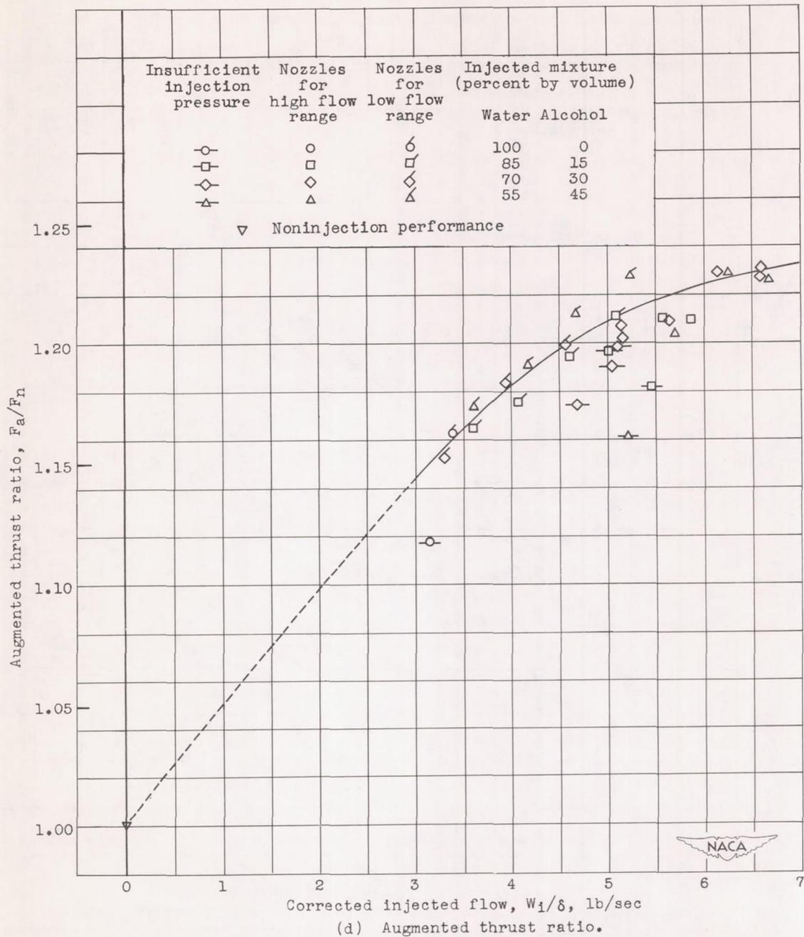
Figure 7. - Concluded. Turbojet-engine performance with three-stage system of water-alcohol injection investigated at sea-level, zero-ram conditions. Data corrected to engine inlet-air temperature of 80° F; engine speed, 7610 rpm; exhaust-gas temperature, 1200° F.
