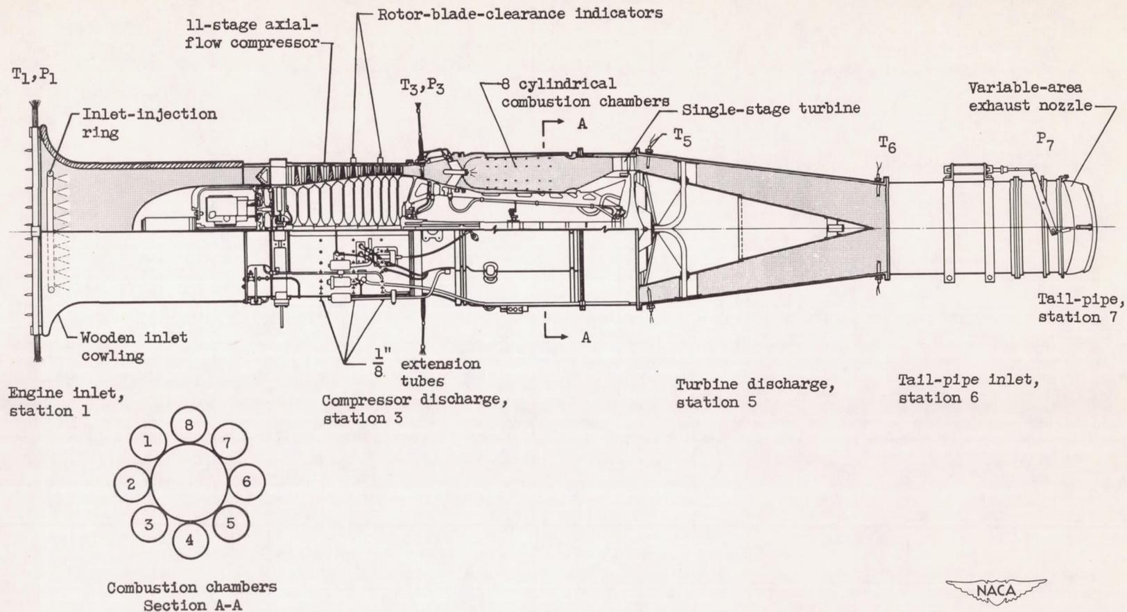
Figure 5. - Engine instrumentation.
