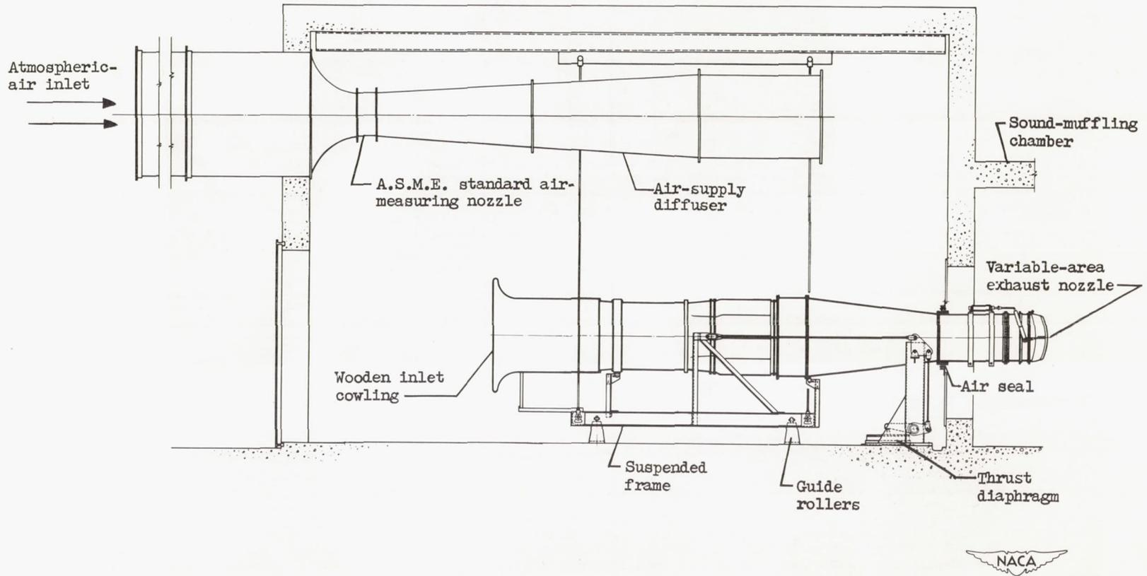
Figure 1. - Schematic diagram of engine installation.
