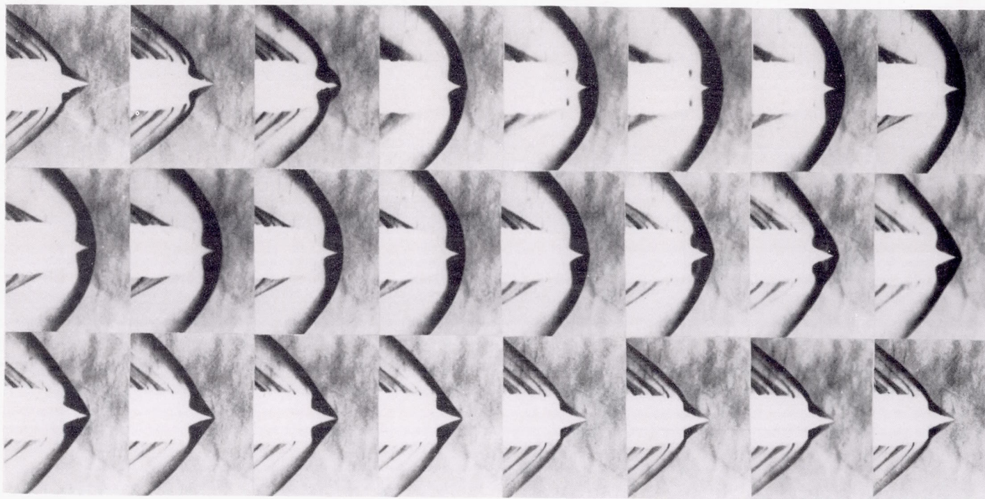
(b) Fuel flow, 78.0 pounds per hour; total-pressure recovery, P_3/P_0 , 0.66; frequency, 28 cycles per second.
