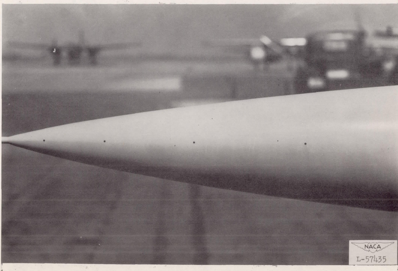
(b) Detail of nose showing body-airspeed-boom juncture and orifices 1 to 4.
