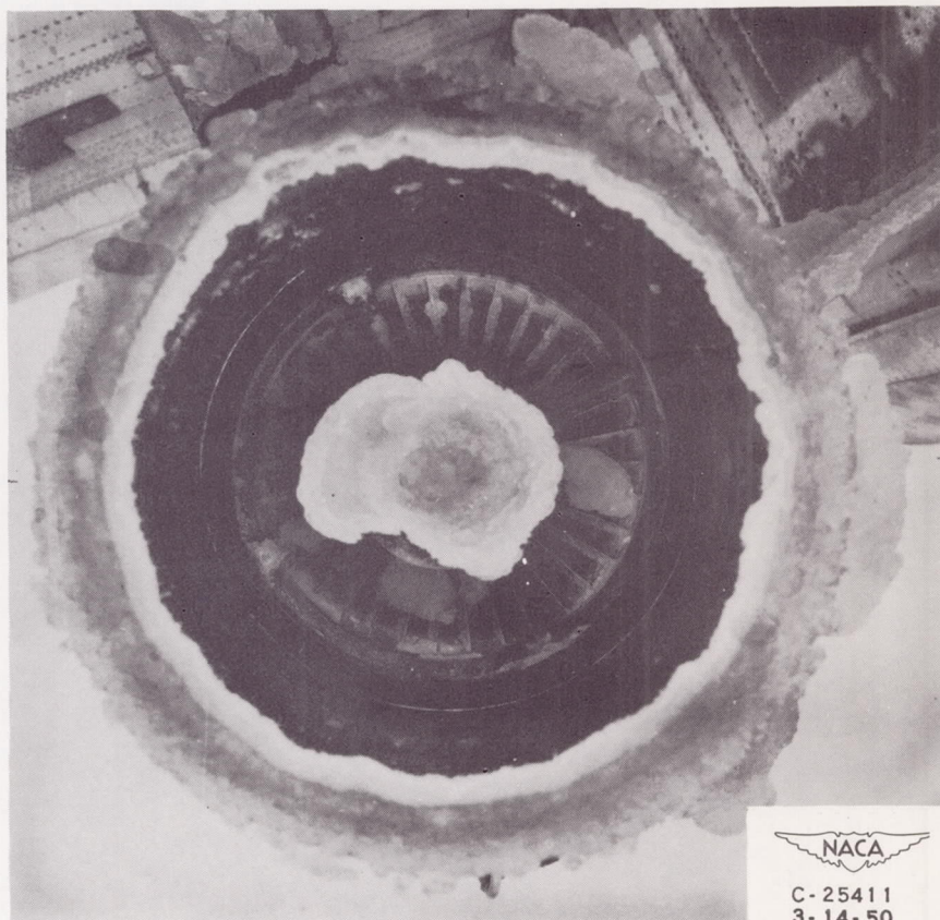
(f) Elapsed time in icing conditions, 47 minutes.
