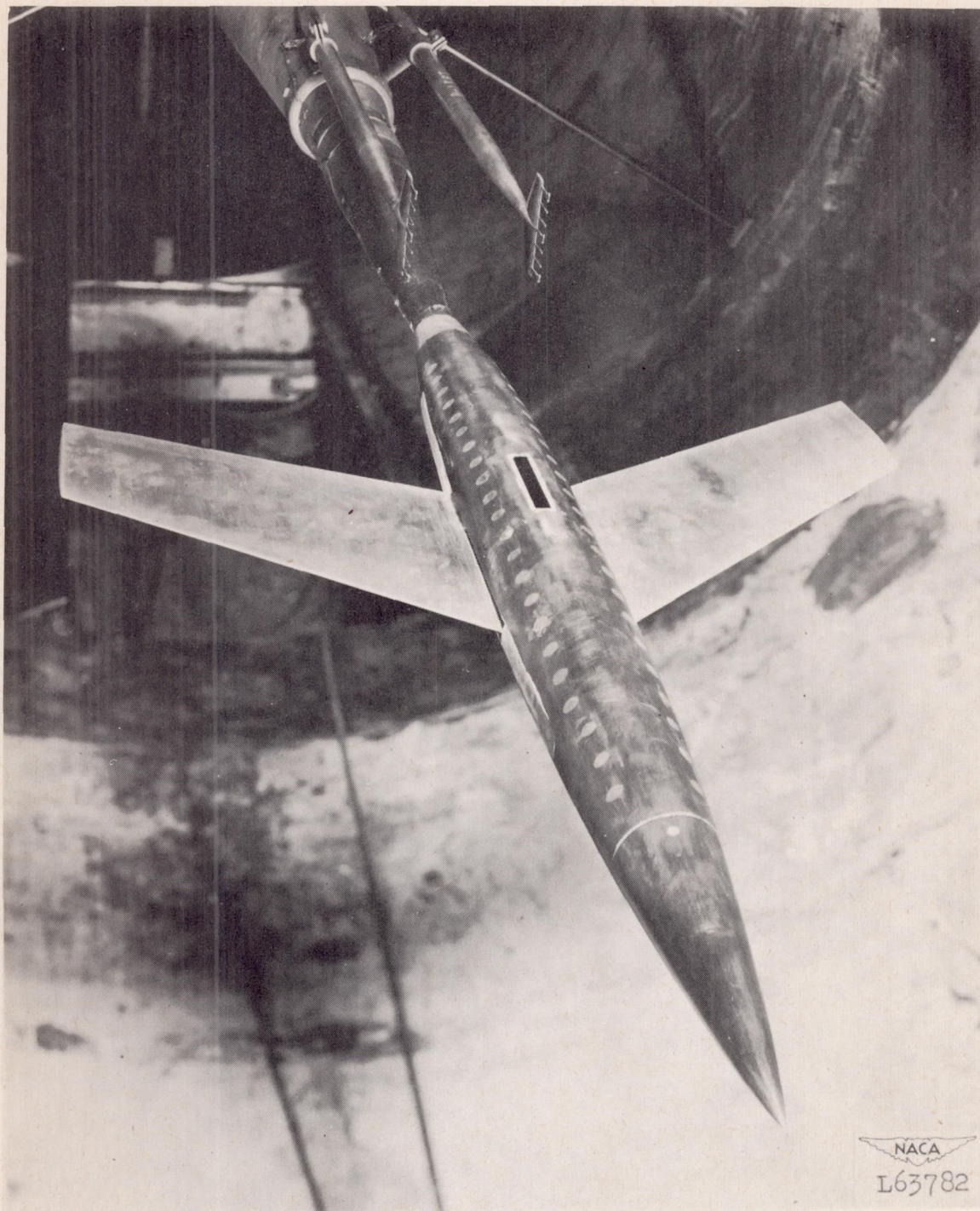
Figure 6.- Photograph of the model in the Langley 8-foot high-speed tunnel.
