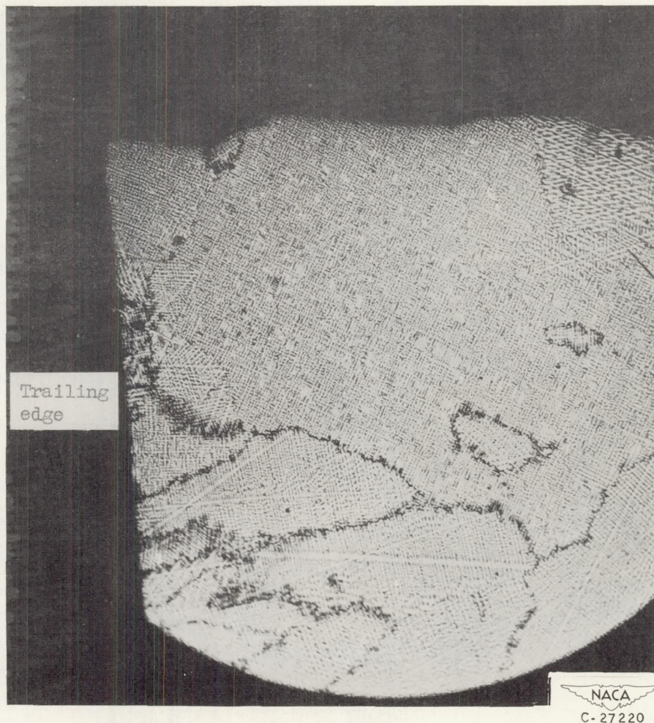
Figure 10. - Transcrystalline path in Stellite 21 fracture blade 25 after 16.75 hours (67 cycles) of operation. Electrolytically etched in 10 percent nitric acid and 10 percent ethylene glycol. X50.
