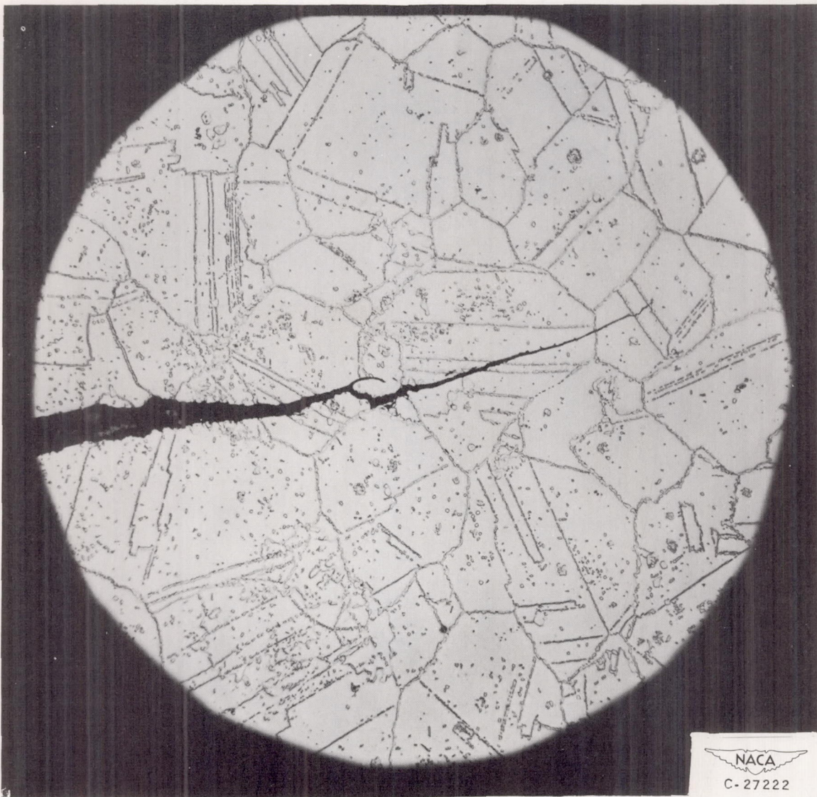
Figure 8. - Transcrystalline trailing-edge crack in Hastelloy B blade 14 after 14.25 hours (57 cycles) of operation. Etchant, aqua regia in glycerine. X250.
