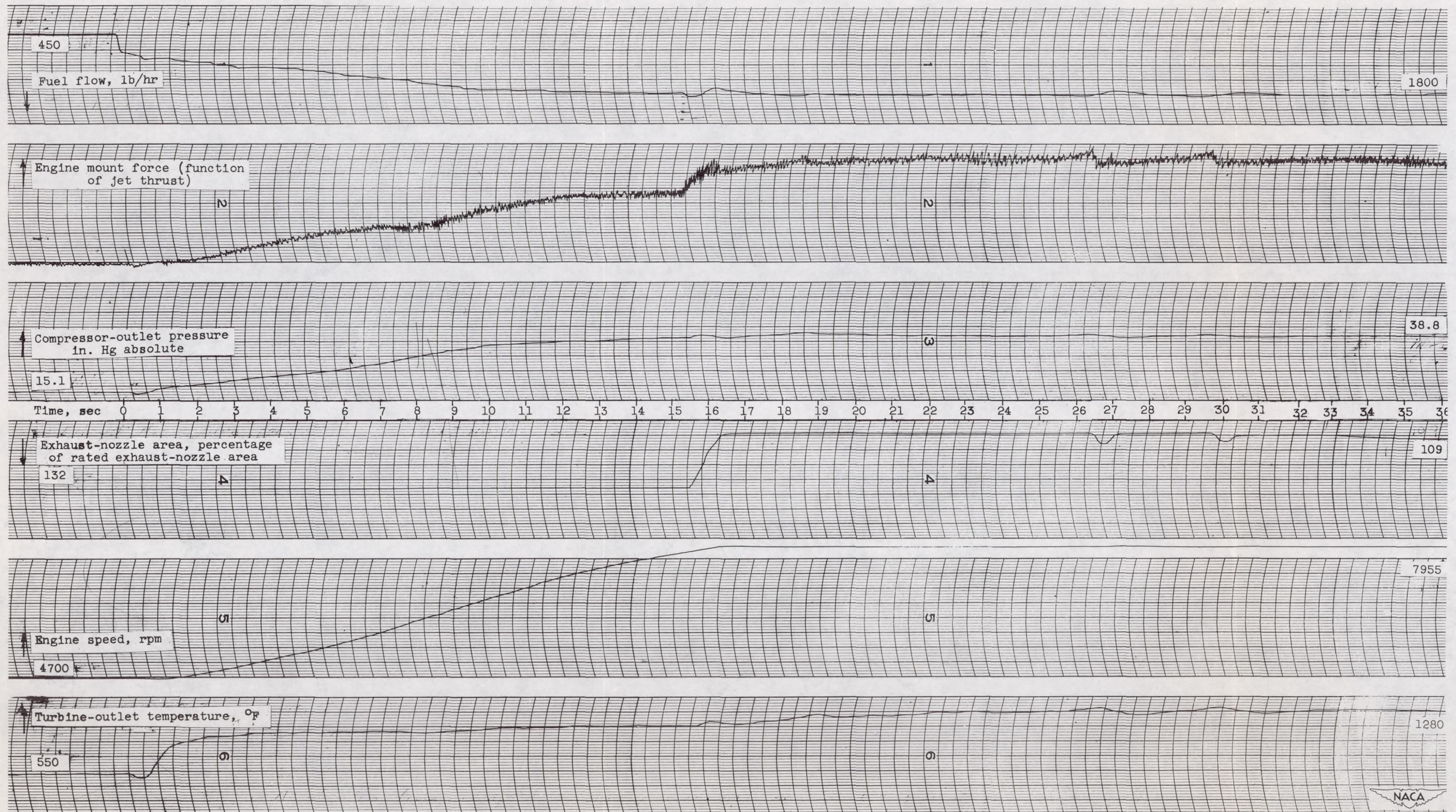
Figure 19. - Throttle-burst acceleration from idle speed to full dry thrust. Altitude, 35,000 feet; flight Mach number, 0.19.
