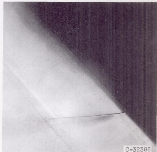
Upper surface. Icing time, 4\frac{1}{2} minutes; section drag coefficient, 0.0115.
