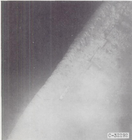
Lower surface. Icing time, 10 minutes; section drag coefficient, 0.0252.
