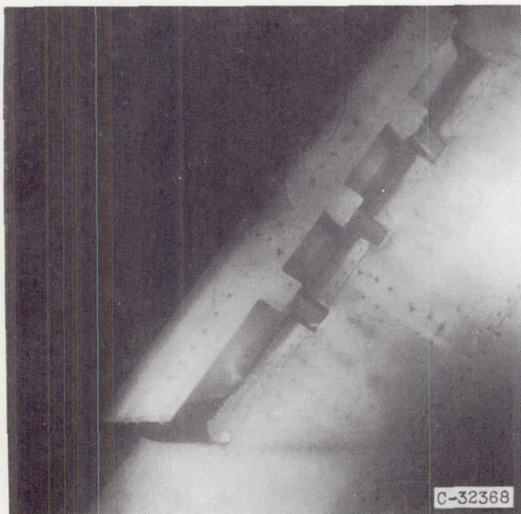
Lower surface. Icing time, 3 minutes; section drag coefficient, 0.0395.
