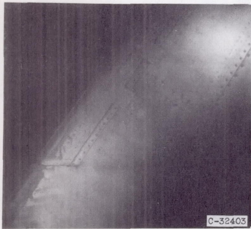
Lower surface. Icing time, 31 minutes; section drag coefficient, 0.0118; standard airfoil; heat-on period, 20 seconds; heat-off period, 460 seconds.
