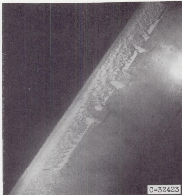
Lower surface. Icing time, 6\frac{1}{2} minutes; section drag coefficient, 0.0160.
