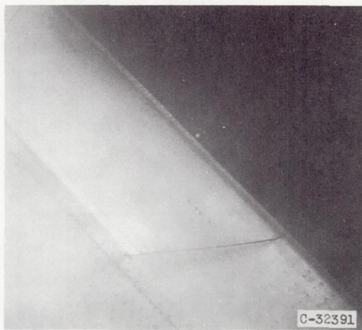
Upper surface. Icing time, 5 minutes; section drag coefficient, 0.0126.
