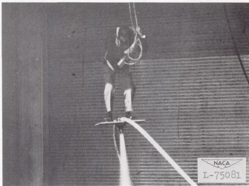
Figure 11.- Flyer B enmeshed in suspension lines at height.
