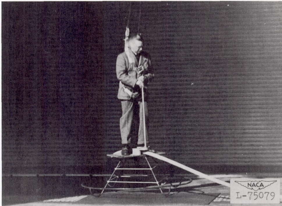
Figure 9.- Control stick installed.
