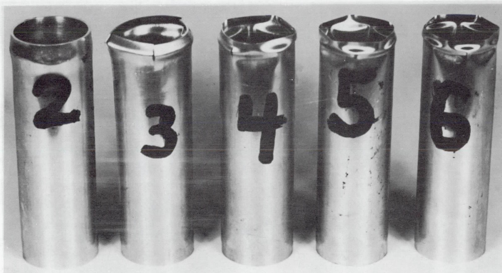
Figure 5.- 75S-T6 specimens after retest under axial compression with original reinforced ends removed.
