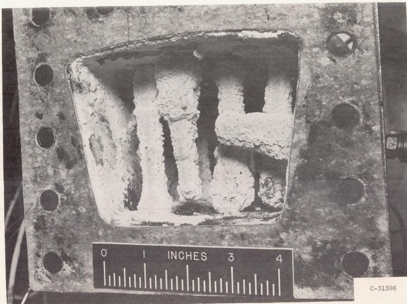
Figure 10. - Deposits on the outlet thermocouples of model 6 combustor.
