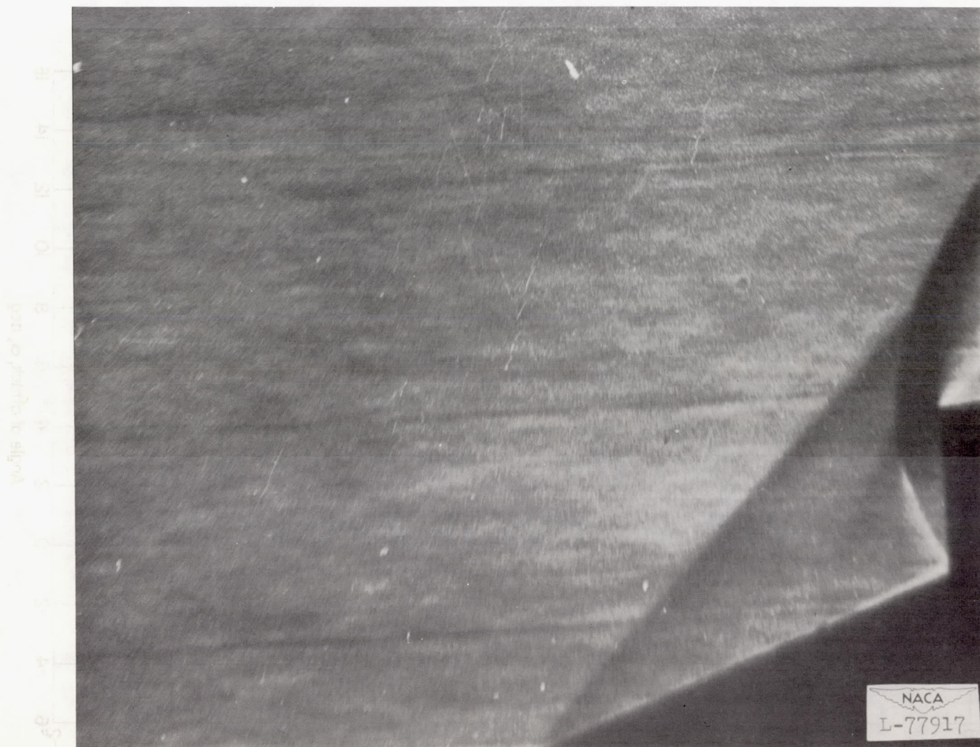
Figure 6.- Schlieren photograph of shock formation at nacelle inlet. \alpha = 0^\circ ; \beta = 0^\circ ; M = 1.61 .
