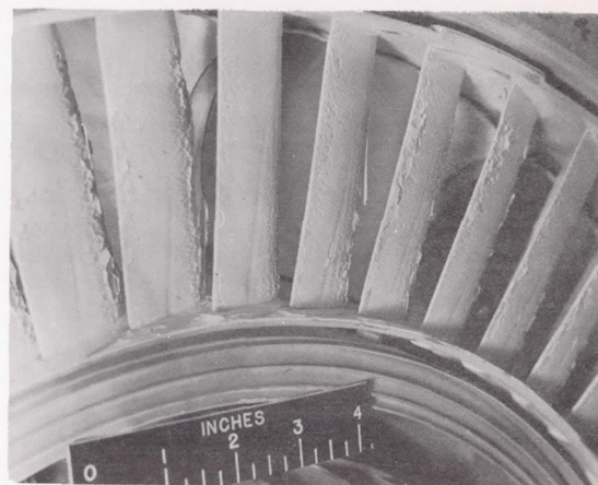
Figure 9. - Stator blades before and after operation with silicone oil, SF-99, added to the fuel.
