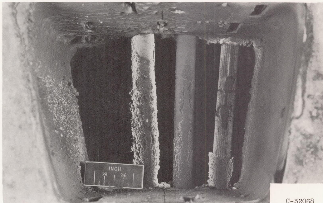
(b) Test condition B; run duration, 2.7 minutes. Combustor-outlet temperature, 1560° F.
