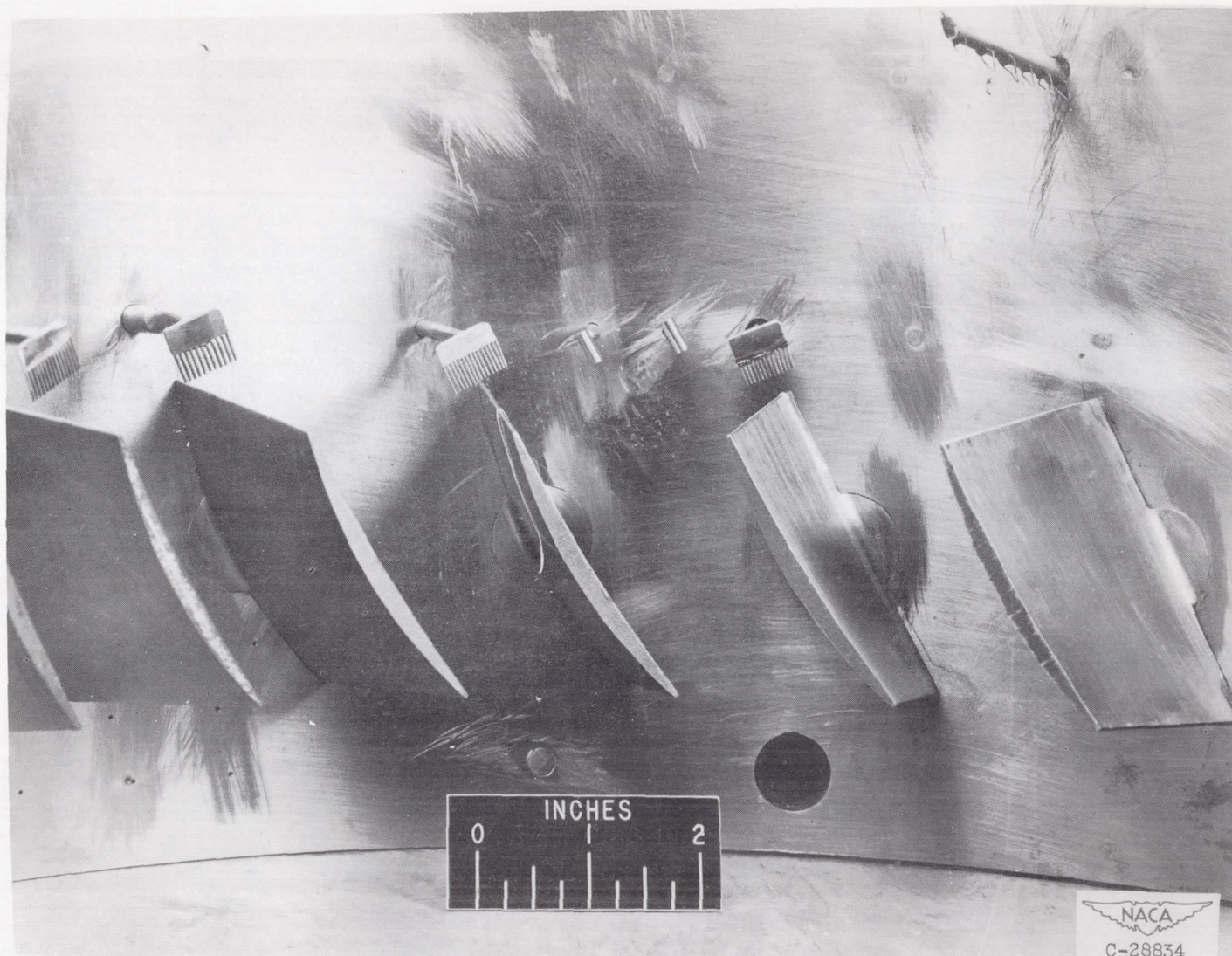
Figure 5. - Location of wake rakes and Kiel probes downstream of stators.
