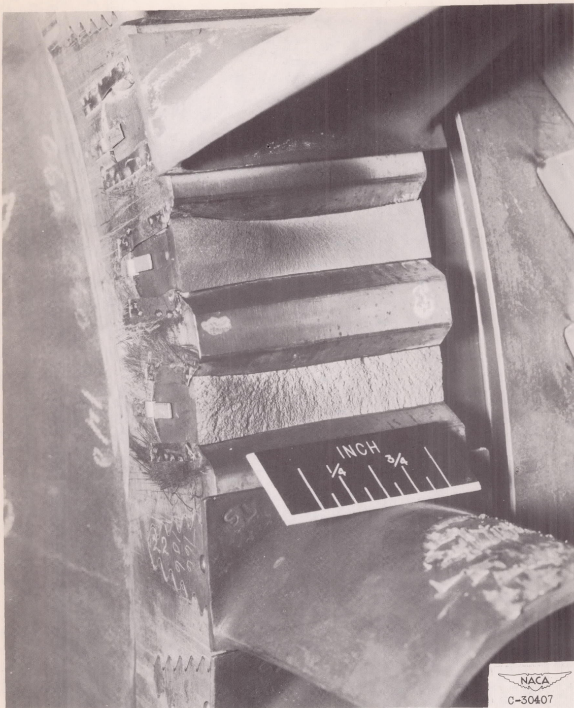
Figure 5. - Root failures in run 12A.
