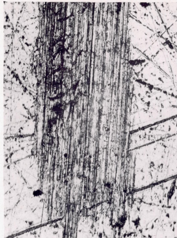
(b) Damage type b, hard slider (hardened steel) against softer plate (SAE 1020 steel); coefficient of friction \mu , 0.79.
