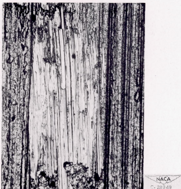
(e) Damage type e, (steel against zirconium); coefficient of friction \mu , 0.44.
