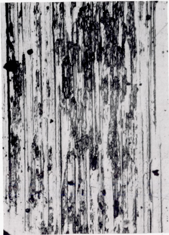
(c) Damage type c, materials of similar hardnesses (monel against stainless steel); coefficient of friction \mu , 0.68.
