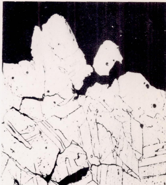
(b) Unaged: failed in 52 hours under a stress of 30,000 psi.
