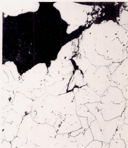
(d) Aged 100 hours at 1600° F: failed in 156 hours under a stress of 20,000 psi.
