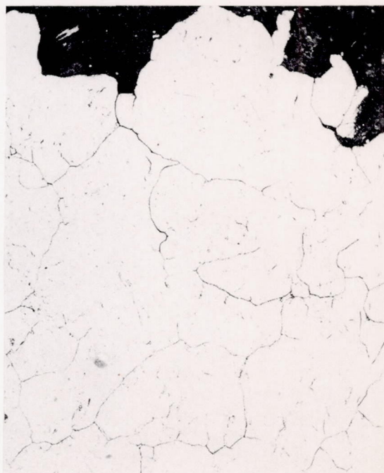
(f) Aged 1000 hours at 1600° F: failed in 53.5 hours under a stress of 65,000 psi.
