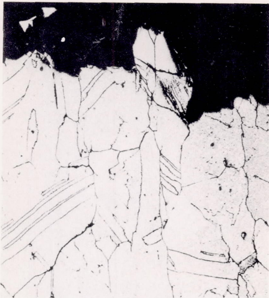
(a) Unaged: failed in 0.61 hour under a stress of 55,000 psi.
