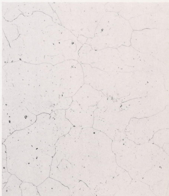
Figure 2.- Microstructure of transverse section of Inconel X bar stock solution-treated 4 hours at 2050° F and water-quenched. Electrolytically etched in 10 percent oxalic acid. X100.
