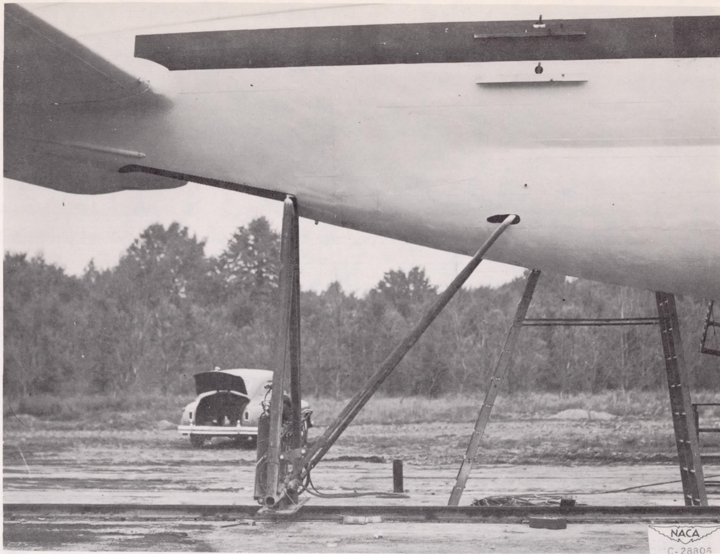
Figure 8. - Extended tail-truss support for holding C-46 airplane in flight attitude.
