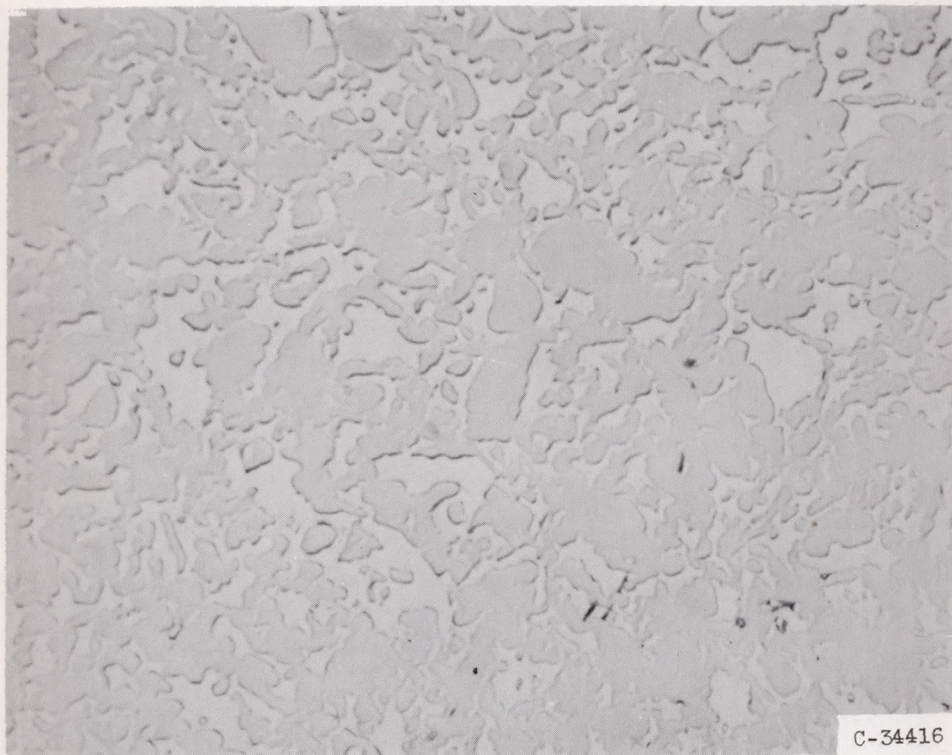
Figure 9. - Photomicrograph of freeze-cast titanium carbide infiltrated with Inconel. X1000
