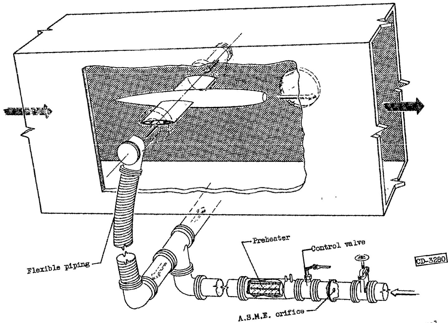
Figure 1. - Schematic diagram of jet-exit model installed in 8- by 6-foot supersonic wind tunnel.
