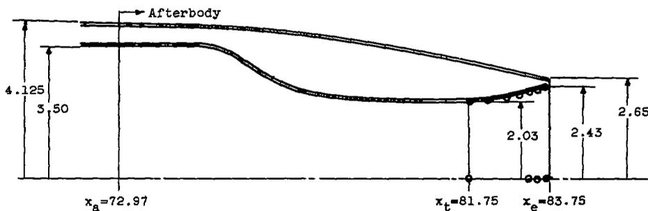
(c) Nozzle 3 (rapid divergent). Design pressure ratio, 5.7.
