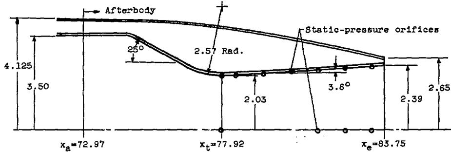
(a) Nozzle 1 (conical element). Design pressure ratio, 5.3.
