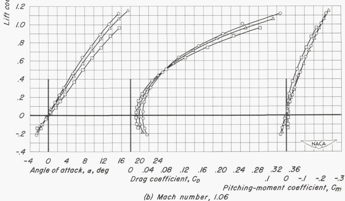
Figure 8.- The lift, drag, and pitching-moment characteristics of the wings.
