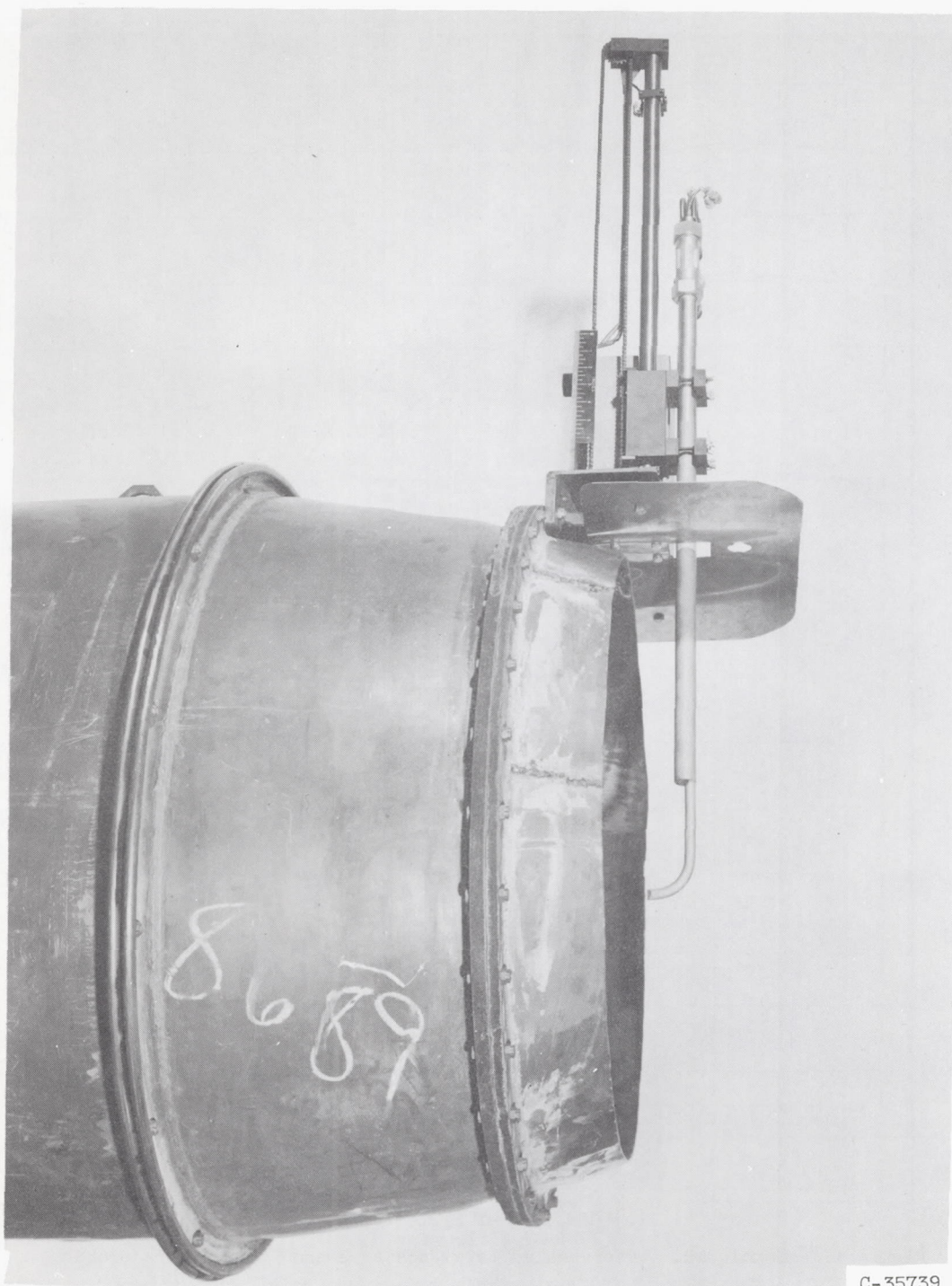
Figure 5. - Probe actuator mounted on afterburner.
