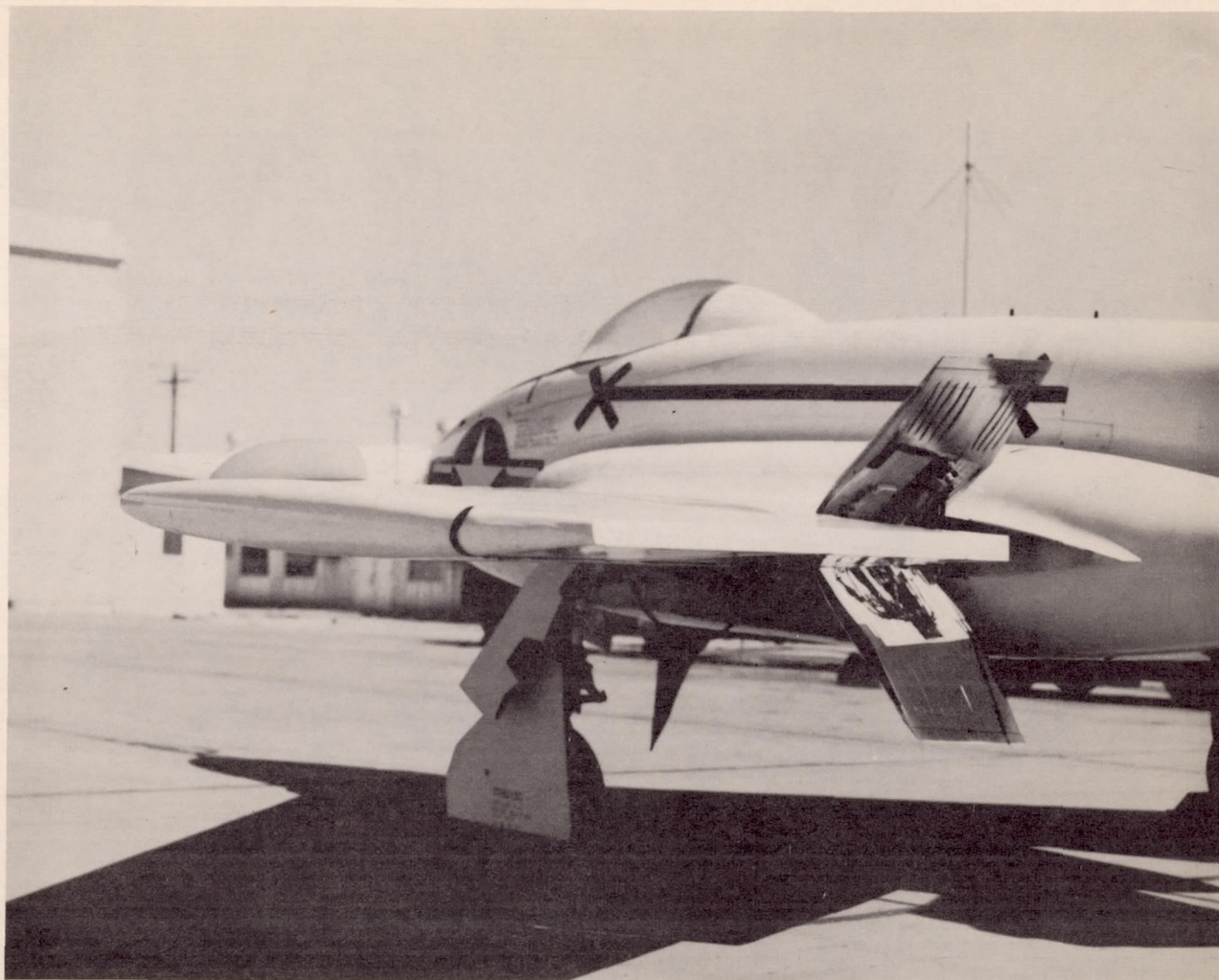
Figure 3.- Photograph of modified elevons of X-4 semitailless airplane.
