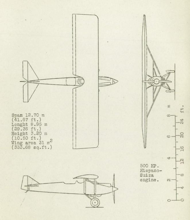
Fig.1 Wibault two-seat all metal monoplane 802.
