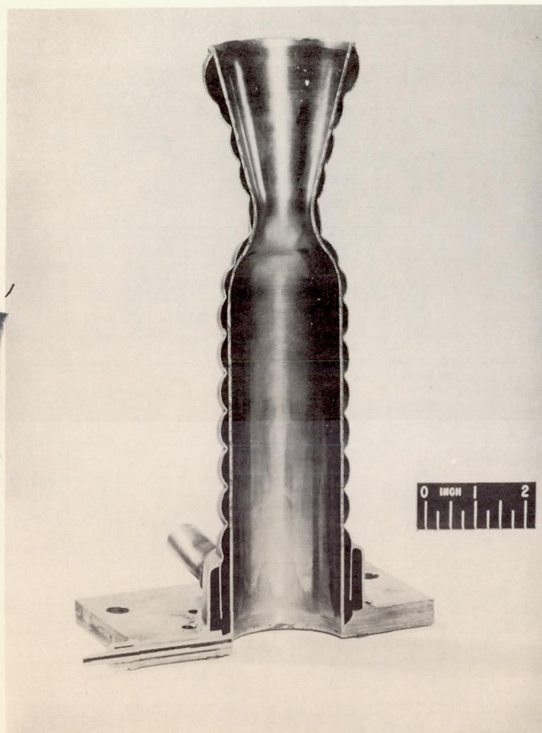
Figure 3. - Cutaway section and diagram of chamber and nozzle of 1000-pound-thrust rocket engine. (Dimensions in inches.)
