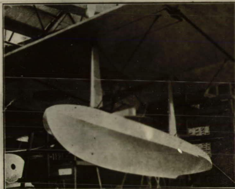
Fig.8 One of the wing-tip floats. Note the pronounced Vee bottom.
