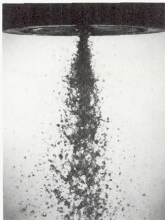
(b) Impinging-jets injector; butt orientation of sprays.
