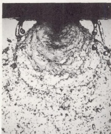
(e) Parallel-sheets injector; parallel orientation of sprays.
