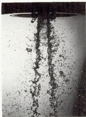
(h) Fuel-sheet - oxidant-jet injector; butt orientation of sprays.
