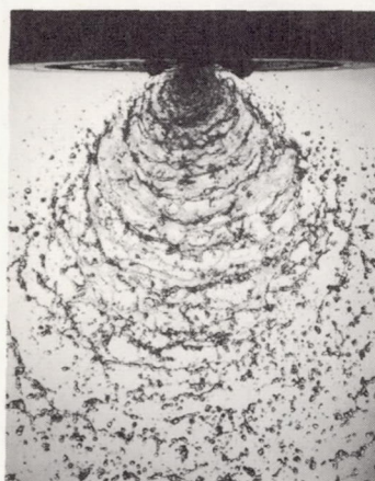
(a) Impinging-jets injector; parallel orientation of sprays.
