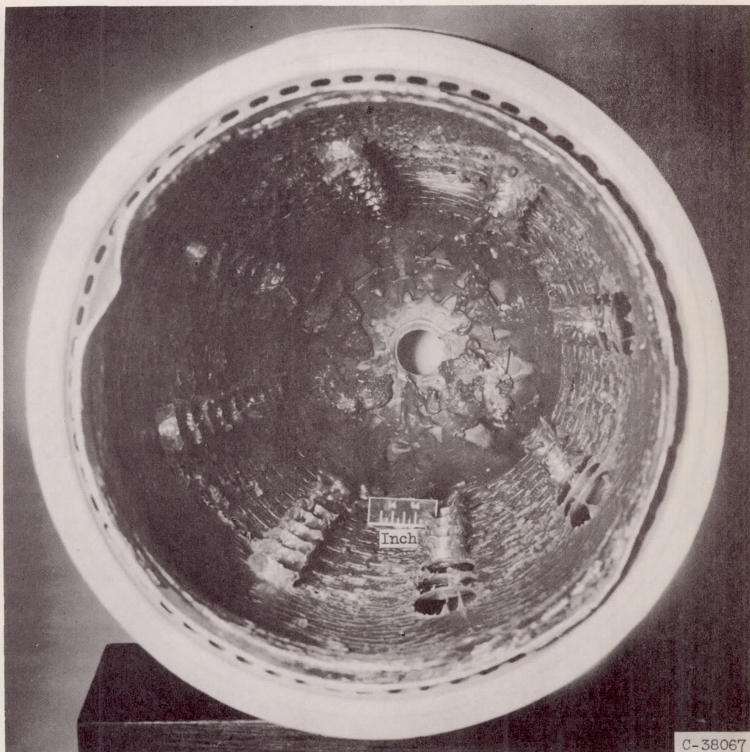
(a) Test 1, combustion chamber with greater deposits. Total test time, 22 minutes.
