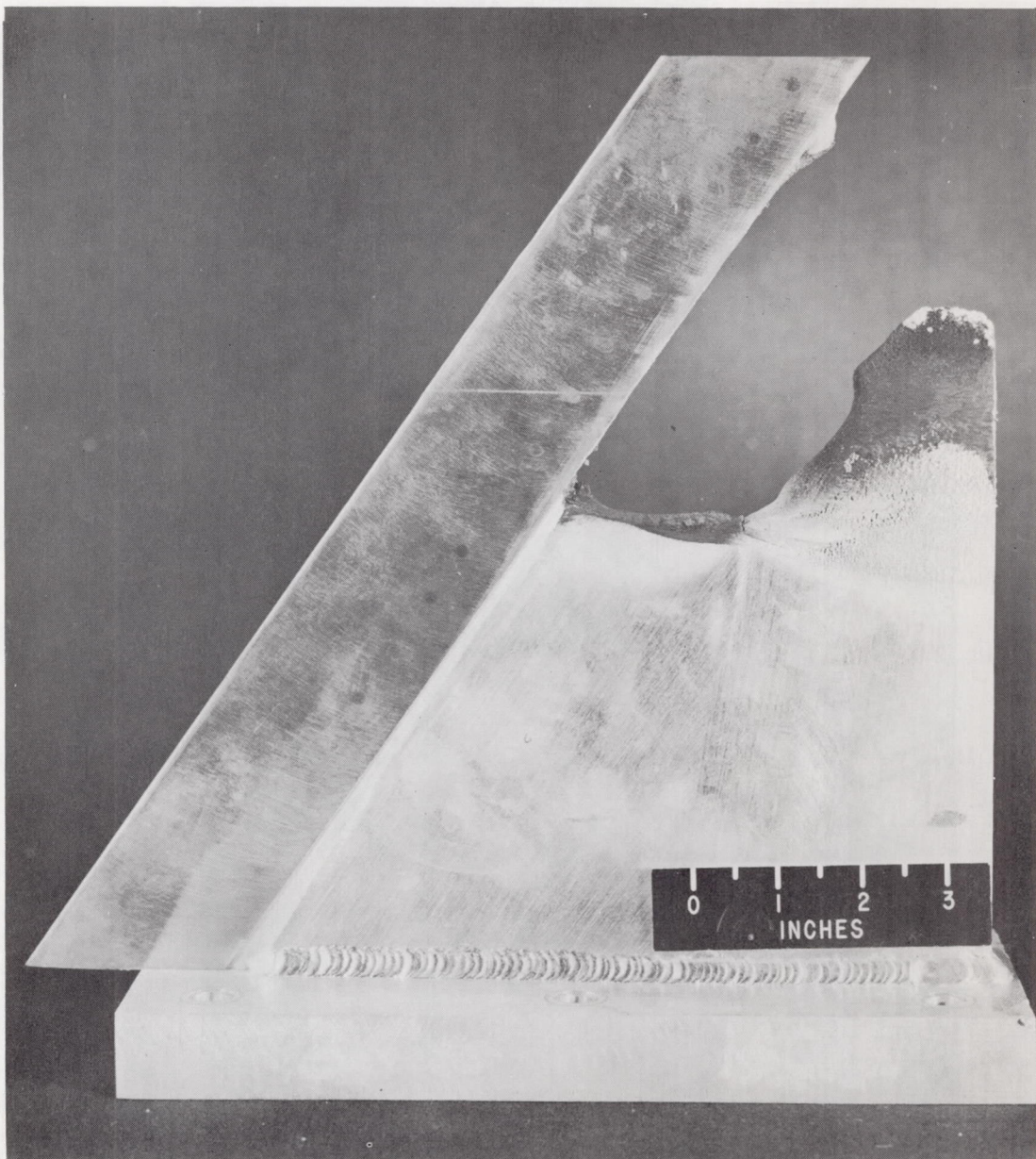
Figure 7.- Damage to model 4 after exposure for 3.7 seconds at 3,500° R.
