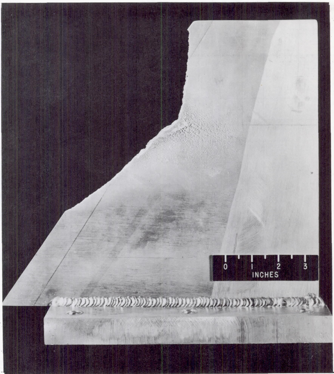
L-93486.1 Figure 4.- Damage to the leading edge of model 1 after exposure for 2.3 seconds at 2,390^{\circ} R.
