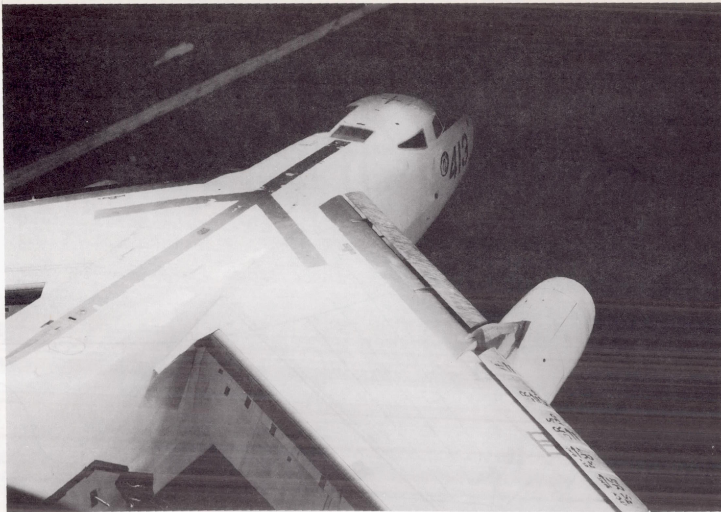
Figure 4.- View from above and behind the right wing showing the test airplane with slat modifications installed over the entire exposed wing leading edges.
