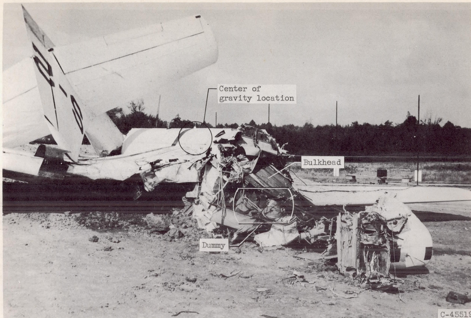
Figure 20. - Extent of damage to fighter airplane after 27^{\circ} unflared landing crash.
