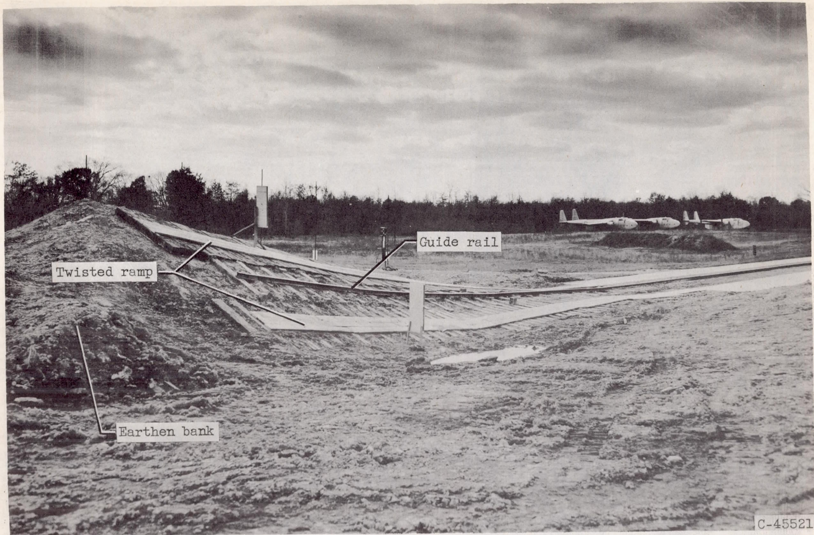
Figure 24. - Ramp designed to cart-wheel airplane entering crash area.
