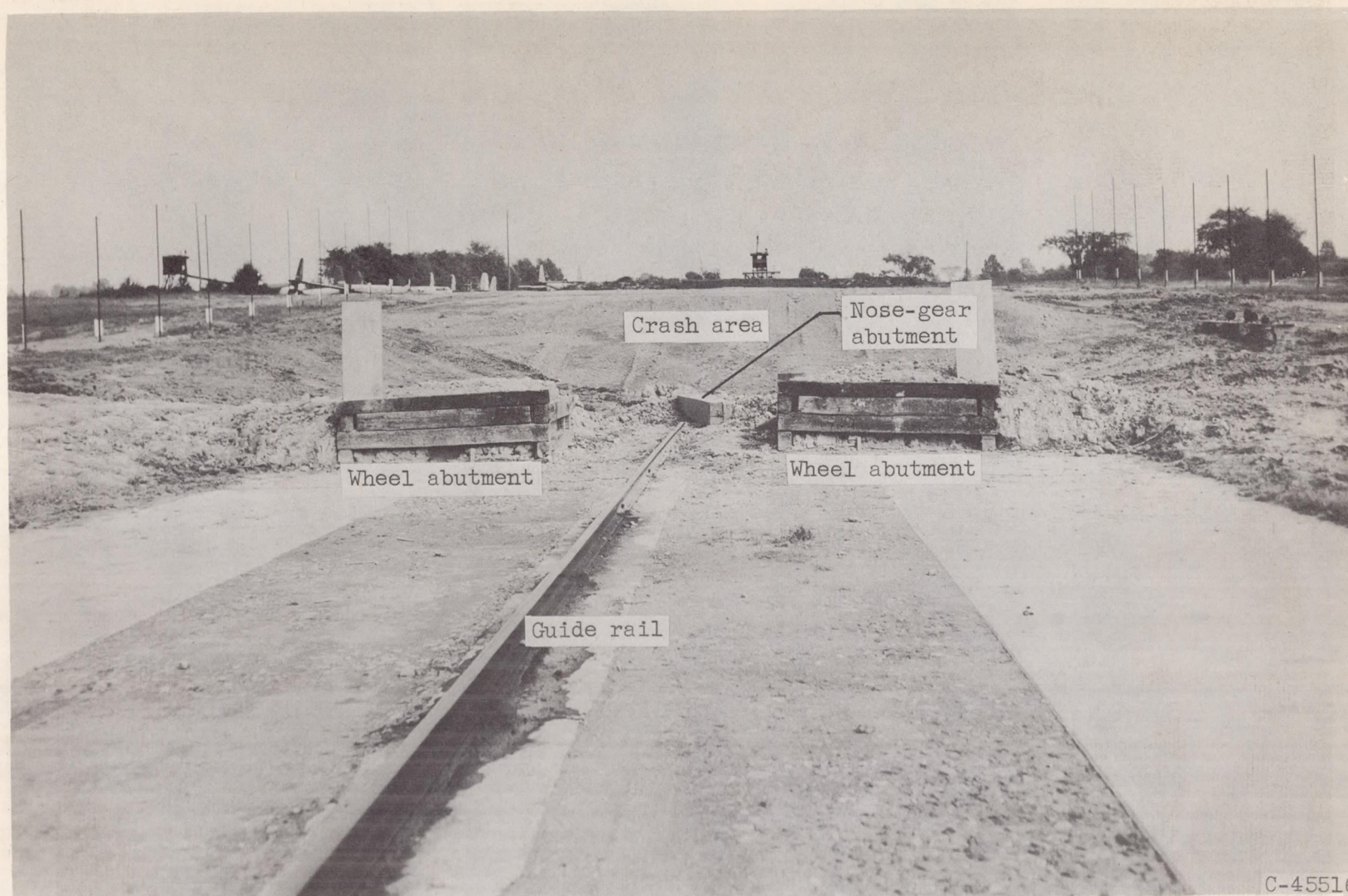
Figure 13. - Crash area used for unflared landing crashes showing wheel and nose-gear abutments.
