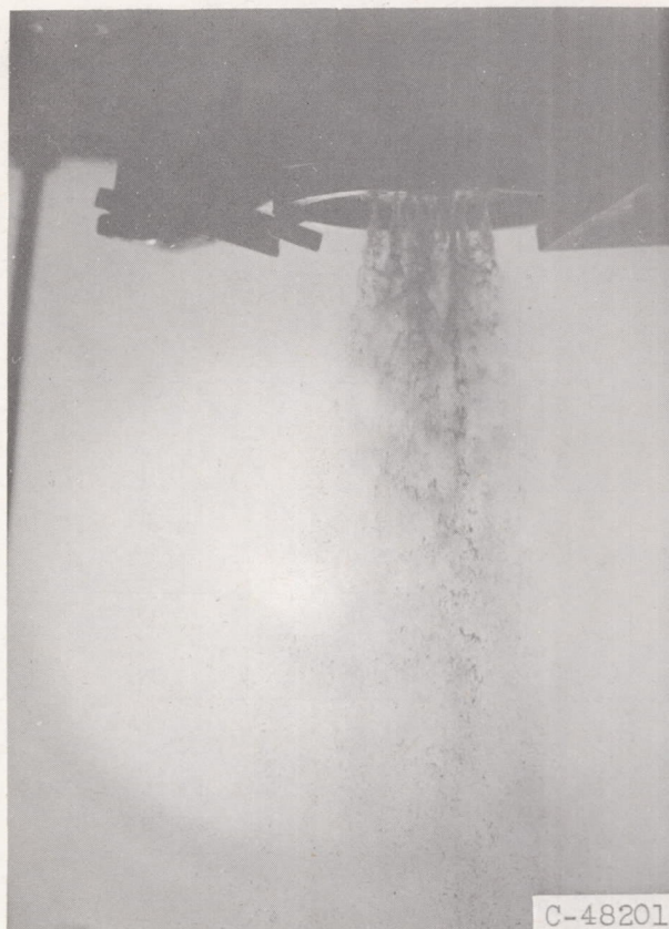
(e) Nine-element configuration. Flow rates: water, 0.370 pound per second; air, 0.058 pound per second.
