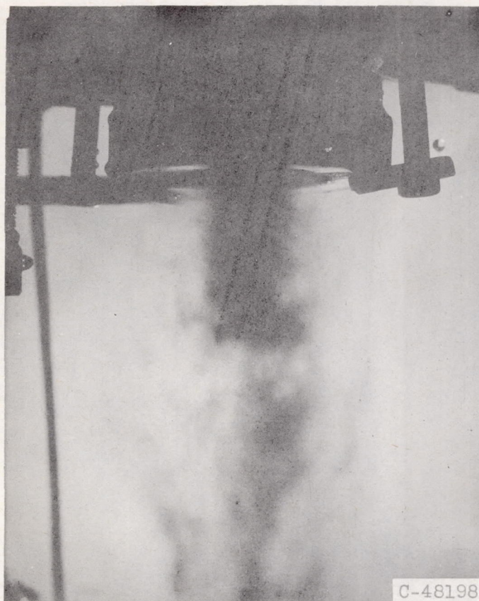
(d) Nine-center-hole plate. Flow rates: water, 0.320 pound per second; air, 0.105 pound per second.
