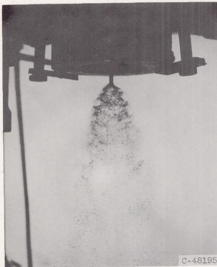
(d) 16-Peripheral-hole plate. Flow rates: water, 0.305 pound per second; air, 0.107 pound per second.
