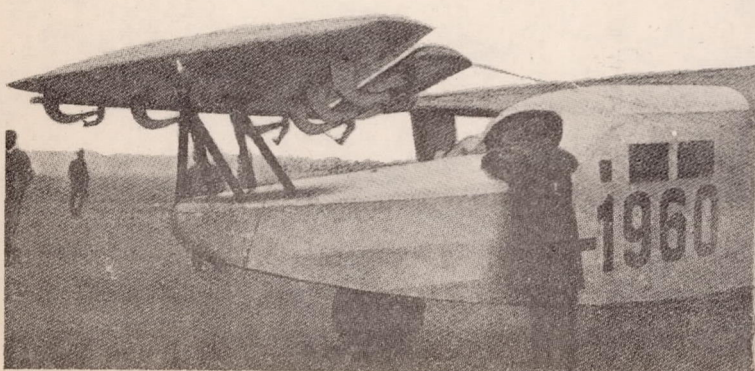
Fig. 4 Three-quarter front view. Note slot arrangement of elevator flaps.
